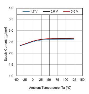
Figure 2. Supply Current vs Ambient Temperature
