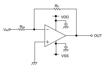
Figure 29. Inverting Amplifier Circuit
