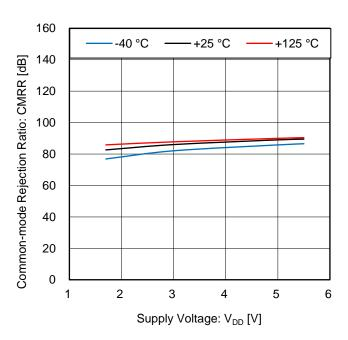
Figure 16. Common-mode Rejection Ratio vs Supply Voltage
