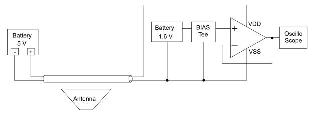
Figure 26. Measurement Circuit of EMI Evaluation
