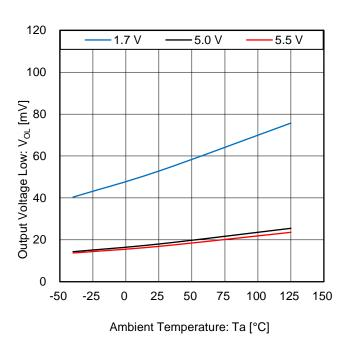
Figure 6. Output Voltage Low vs Ambient Temperature (Iout = 1 mA)
