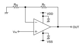
Figure 30. Non-inverting Amplifier Circuit
