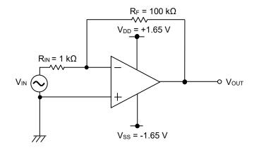
$$V_{OUT} = -\frac{R_F}{R_{IN}} V_{IN}$$
