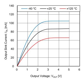
Figure 9. Output Sink Current vs Output Voltage (V<sub>DD</sub> = 5 V)
