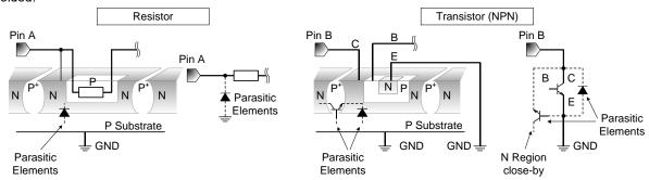
Figure 31. Example of Monolithic IC Structure
