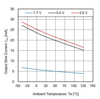
Figure 10. Output Sink Current vs Ambient Temperature (V<sub>OUT</sub> = V<sub>SS</sub> + 0.4 V)
