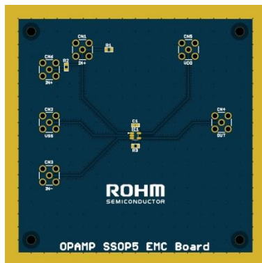
Figure 22. EMI Evaluation Board (BD87521YG-C)
