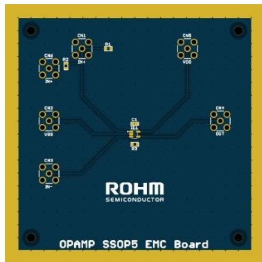
Figure 22. EMI Evaluation Board (BD87521G-LB)
