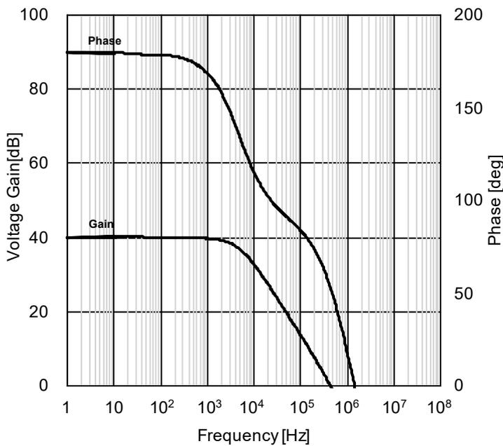
Figure 47. Voltage Gain · Phase vs Frequency (VDD=+3V, VSS=0V, T<sub>A</sub>=25°C)
