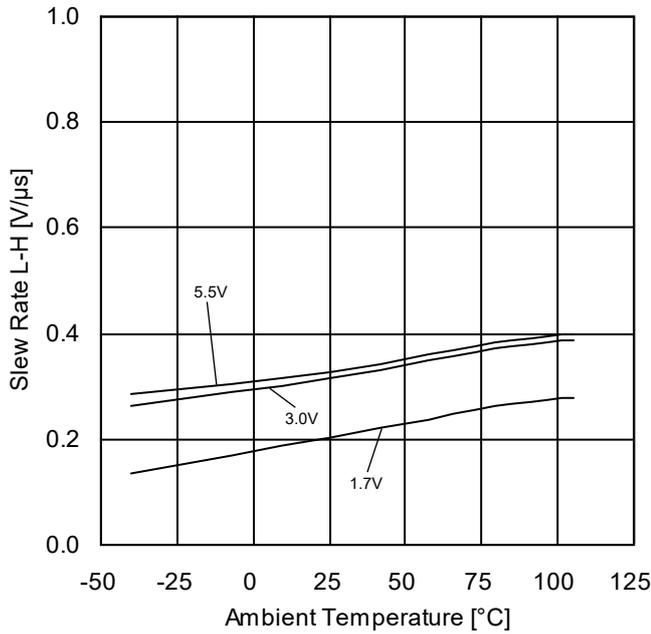
Figure 45. Slew Rate L-H vs Ambient Temperature
