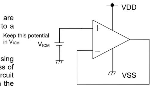
Figure 79. Example of Application Circuit for Unused Op-amp
