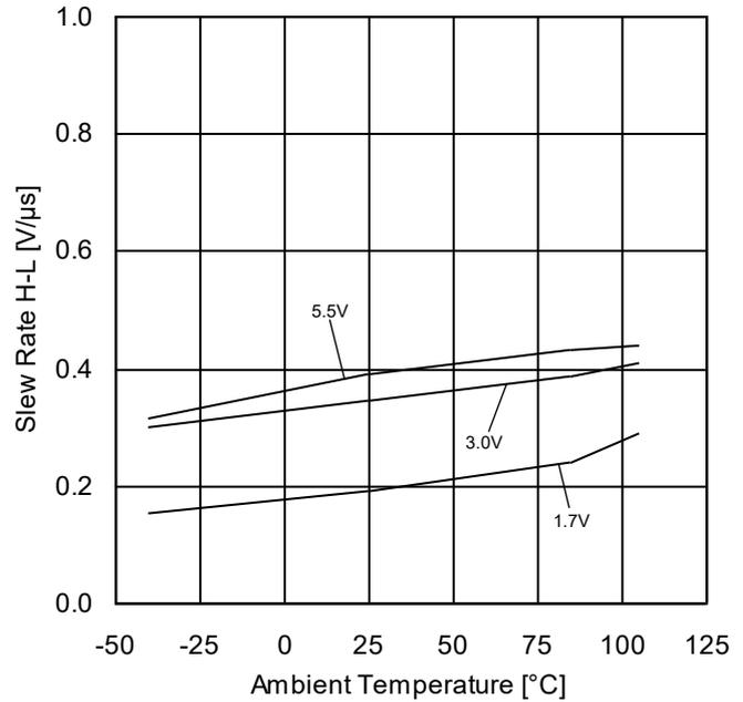
Figure 46. Slew Rate H-L vs Ambient Temperature
