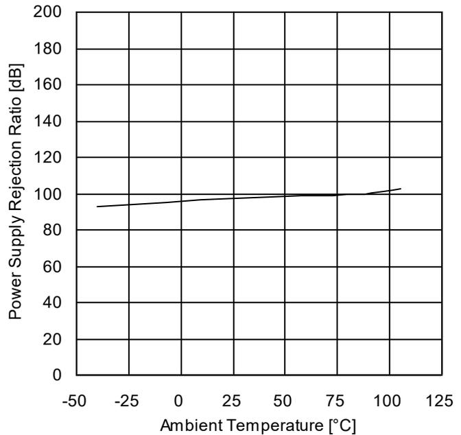
Figure 21. Power Supply Rejection Ratio vs Ambient Temperature
