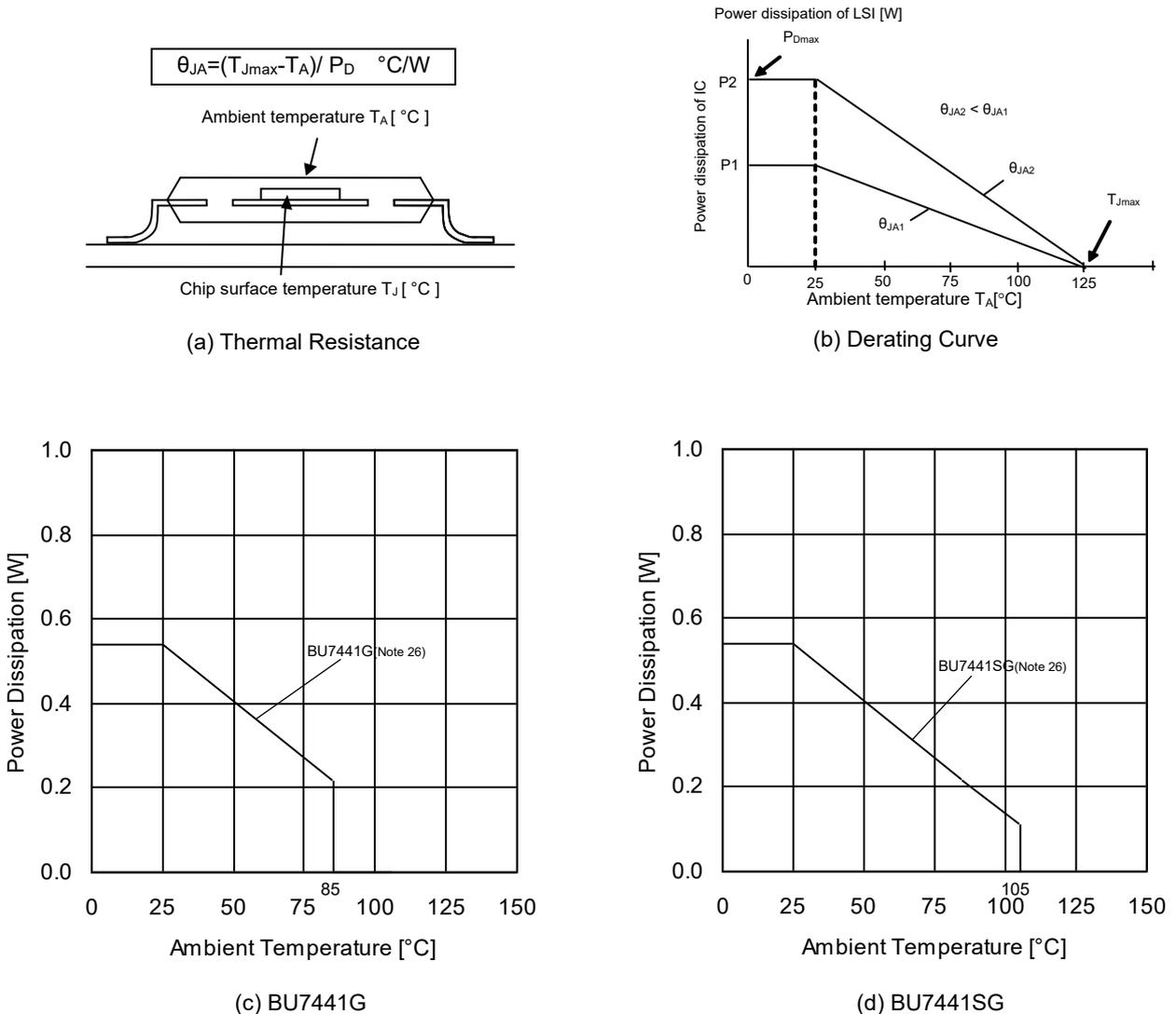
Figure 78. Thermal Resistance and Derating Curve
