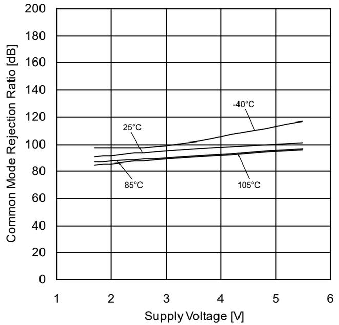
Figure 19. Common Mode Rejection Ratio vs Supply Voltage
