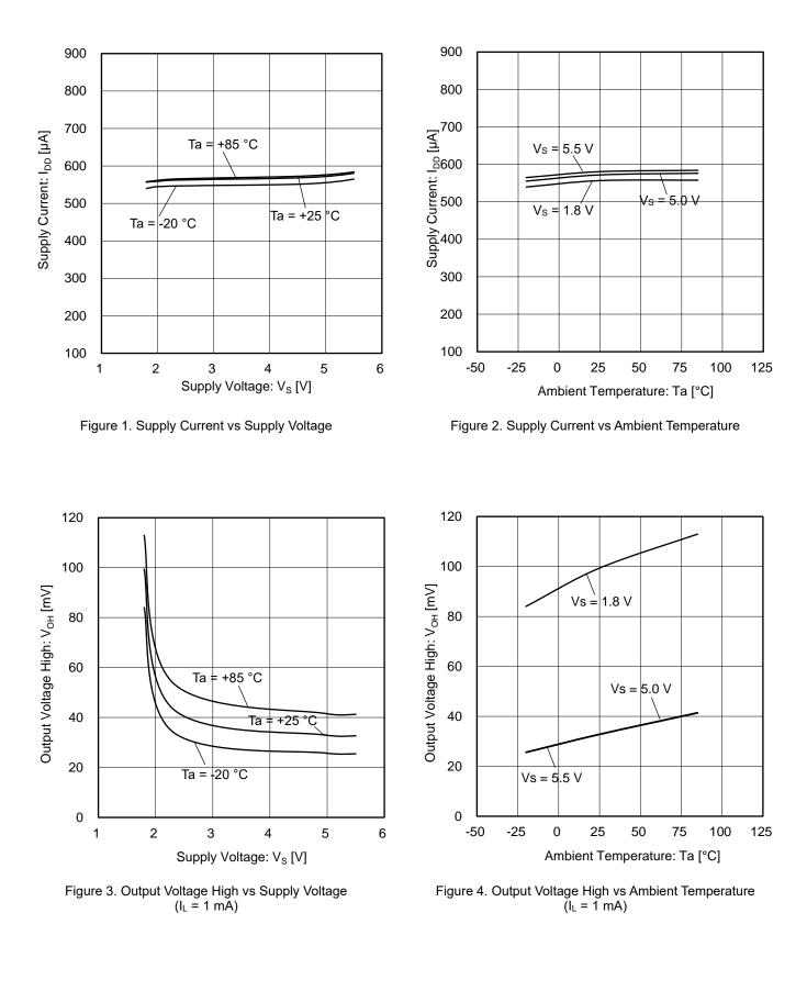
(Note) The above data is measurement value of typical sample, it is not guaranteed.
