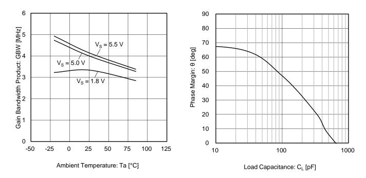
Figure 21. Gain Bandwidth Product vs Ambient Temperature
