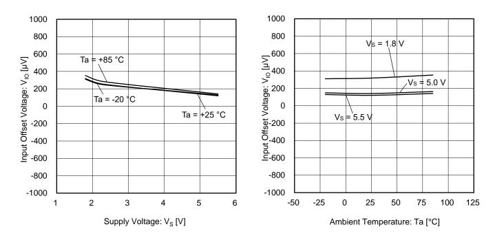
Figure 9. Input Offset Voltage vs Supply Voltage
