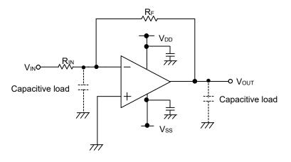
Figure 30. Example of capacitive load
