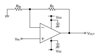
Figure 33. Non-inverting Amplifier Circuit
