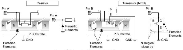
Figure 34. Example of Monolithic IC Structure
