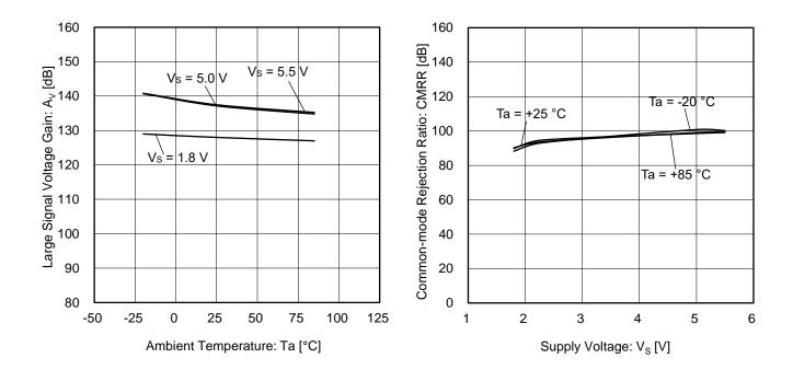
Figure 13. Large Signal Voltage Gain vs Ambient Temperature
