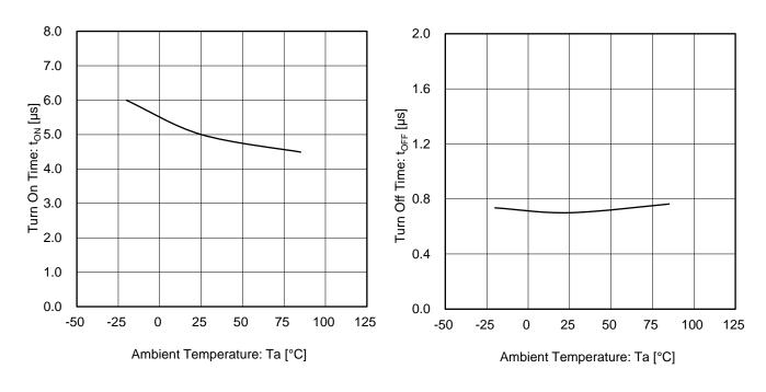
Figure 25. Turn On Time vs Ambient Temperature  $(V_S = 5 V)$
