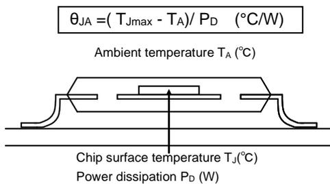
Figure 7. Thermal resistance
