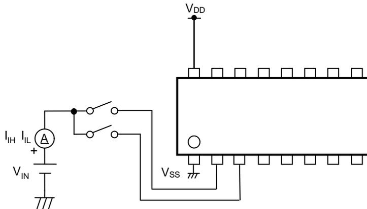
Figure 4. Test Circuit of Input H/L Current
