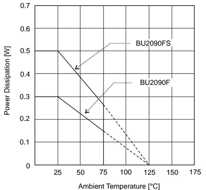
Figure 8. Derating Curve
