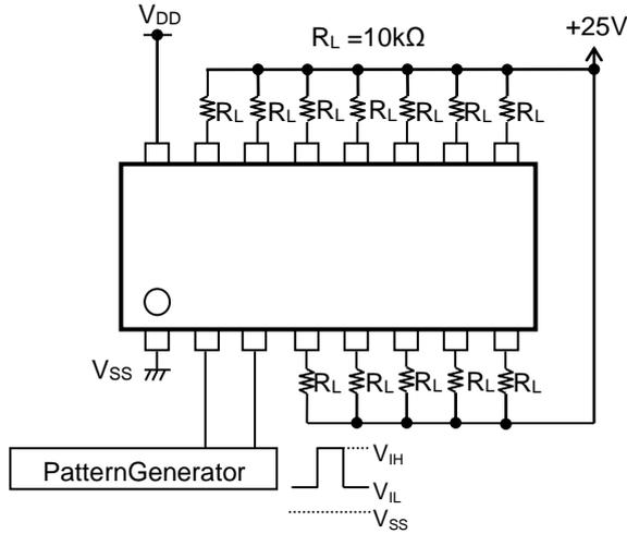
Figure 2. Test Circuit of Input H/L Voltage
