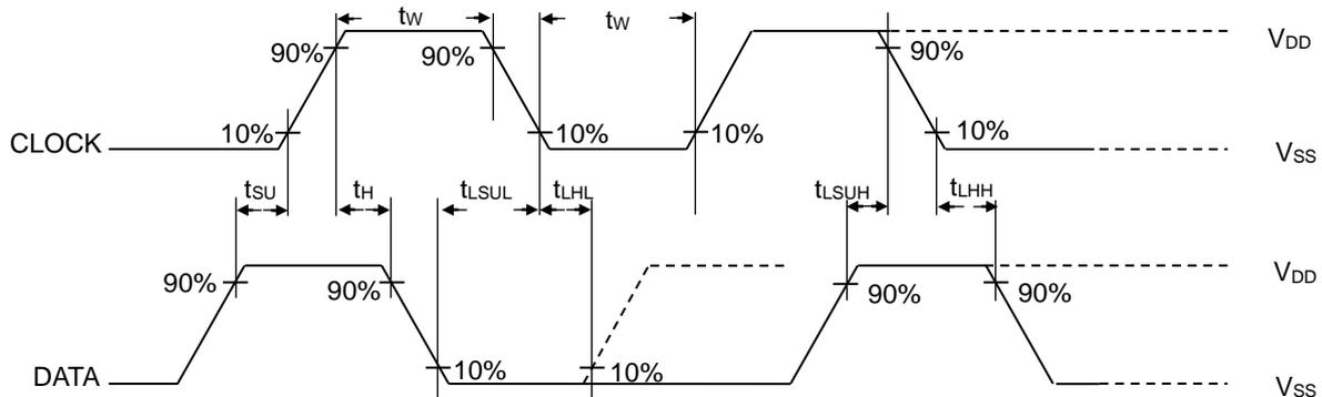
Figure 1. Waveform of Timing Characteristics
