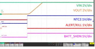
Figure 21. Start Up through NTC Pin
