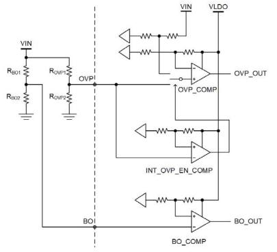
Figure 44. Circuit Diagram around OVP, BO Setting
