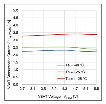
Figure 7. VBAT Consumption Current 3 vs VBAT Voltage
