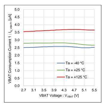
Figure 5. VBAT Consumption Current 1 vs VBAT Voltage
