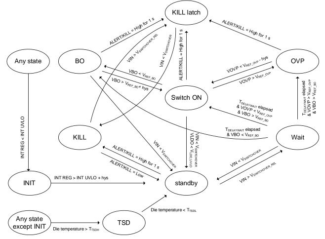
Figure 29. State Transition Diagram
