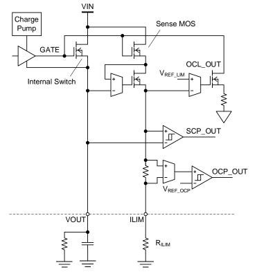
Figure 45. Circuit Diagram around OCL Setting
