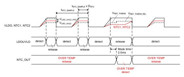
Figure 32. Timing Chart of Burst Operation LDO (When VBAT only supplied)
