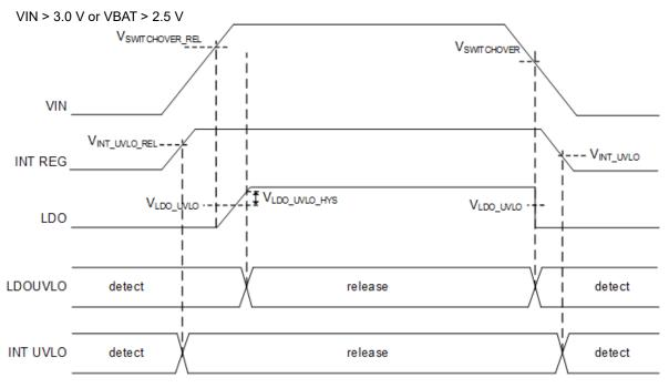
Figure 31. LDO UVLO Detection, Release Condition
