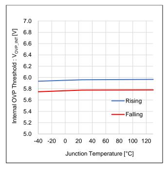
Figure 8. Internal OVP Threshold vs Temperature
