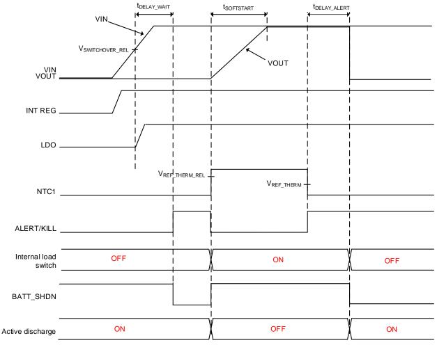
Figure 34. Timing Chart when use NTC1 as EN
