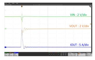
Figure 26. Short Circuit Protection Response
