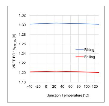
Figure 11. VREF BO vs Temperature
