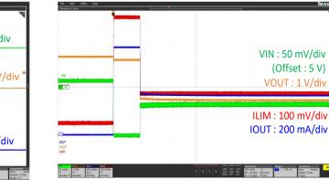
Figure 28. OCL Function (OCL = 500 mA Setting)
