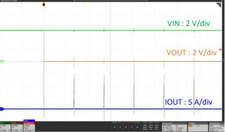
Figure 27. Short Circuit Protection Response (Zoom out)
