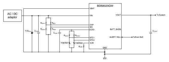
Figure 47. Application Circuits of AC/DC Adapter System Configuration
