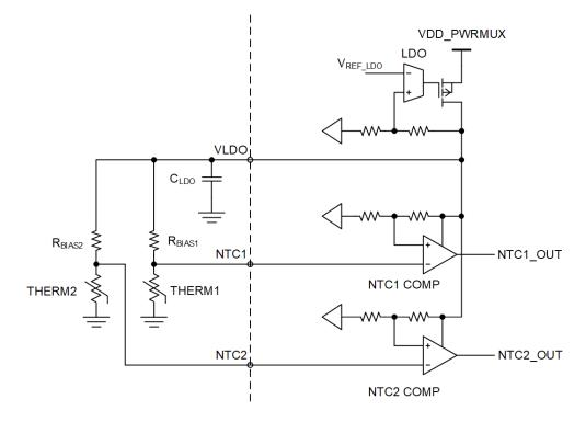
Figure 43. Circuit Diagram around Over Temperature Protection Setting
