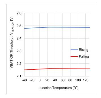
Figure 14. VBAT OK Threshold vs Temperature
