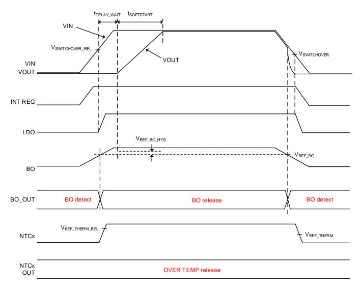
Figure 30. Startup and shutdown sequence when VIN only supplied
