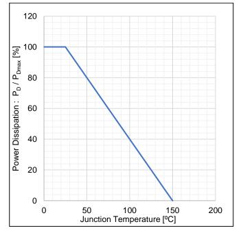
Figure 18. Derating Curve for SOA
