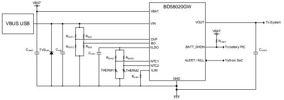
Figure 46. Application Circuits of USB and Battery Configuration
