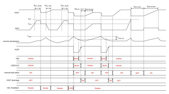
Figure 37. Over Current Limit Function and Over Current Protection Function Timing Chart
