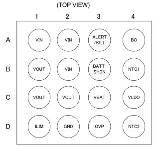
Figure 2. Pin Configuration (TOP VIEW)
