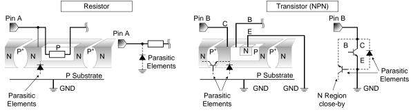
Figure 48. Example of Monolithic IC Structure
