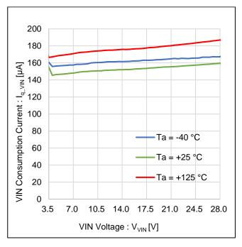
Figure 4. VIN Consumption Current vs VIN Voltage
