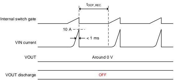
Figure 38. Short Circuit Protection Timing Chart
