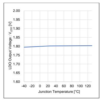
Figure 16. LDO Output Voltage vs Temperature
