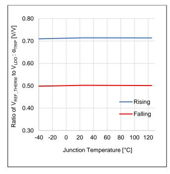
Figure 12.  $\alpha_{TRIP}$  (V<sub>REF\_THERM</sub> / V<sub>LDO</sub>) vs Temperature
