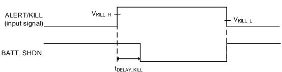
Figure 41. KILL Function (When VIN is below VSWITCHOVER) Timing Chart
