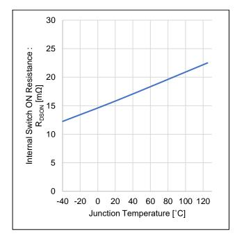
Figure 15. Internal Switch ON Resistance vs Temperature
