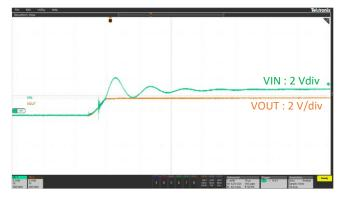
Figure 25. OVP Response (OVP Pin = GND)
