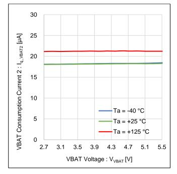
Figure 6. VBAT Consumption Current 2 vs VBAT Voltage
