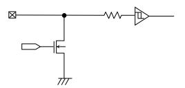
Figure 57. Input/Output Pin Circuit Diagram (SDA)
