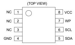
Figure 3-(a). Pin Configuration (SOP-J8, TSSOP-B8, MSOP8)
