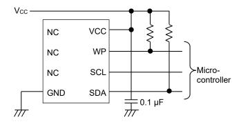
Figure 1. Typical Application Circuit
