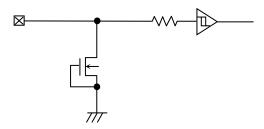
Figure 56. Input Pin Circuit Diagram (SCL)
