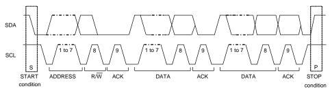
Figure 39. Data Transfer Timing
