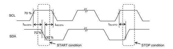
Figure 5-(b). Start-Stop Condition Timing
