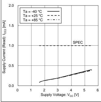
Figure 13. Supply Current (Read) vs Supply Voltage (f<sub>SCL</sub> = 1 MHz)
