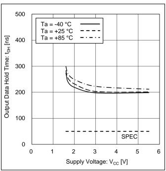
Figure 27. Output Data Hold Time vs Supply Voltage (SDA 'LOW' to 'HIGH')
