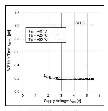
Figure 36. WP Hold Time vs Supply Voltage
