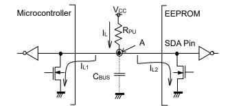
Figure 49. I/O Circuit Diagram
