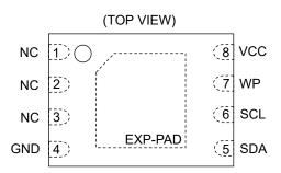
Figure 3-(b). Pin Configuration (VSON008X2030)
