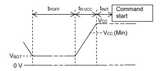
Figure 54. Rise Waveform Diagram
