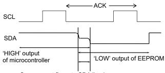
Over current flows to SDA line by 'HIGH' output of microcontroller and 'LOW' output of EEPROM.
