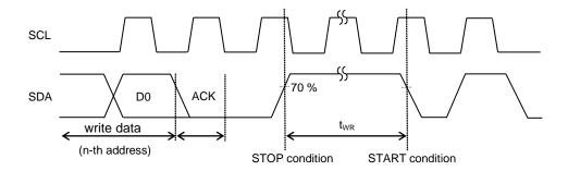
Figure 5-(c). Write Cycle Timing
