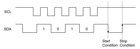
Figure 48. The Case of Cancel by Start, Stop Condition during Target Address Input
