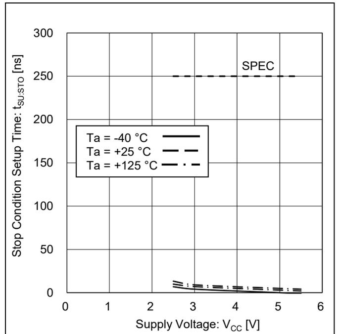
Figure 29. Stop Condition Setup Time vs Supply Voltage
