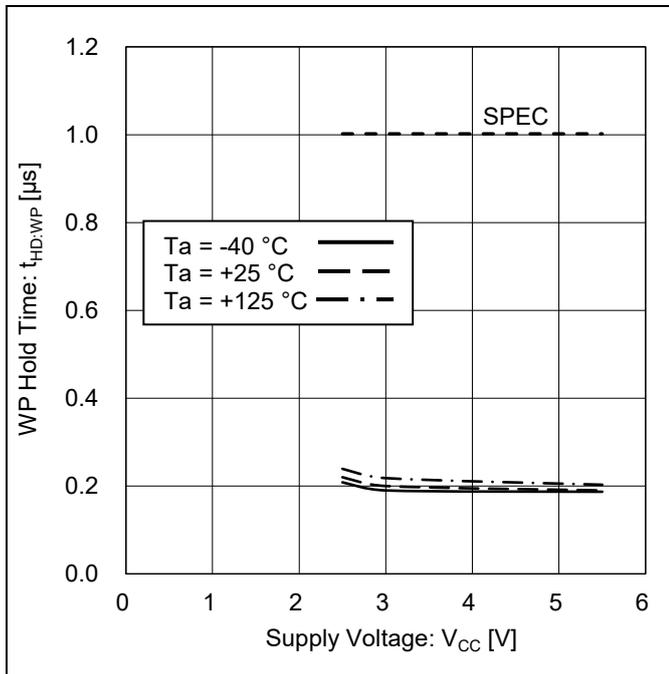
Figure 36. WP Hold Time vs Supply Voltage
