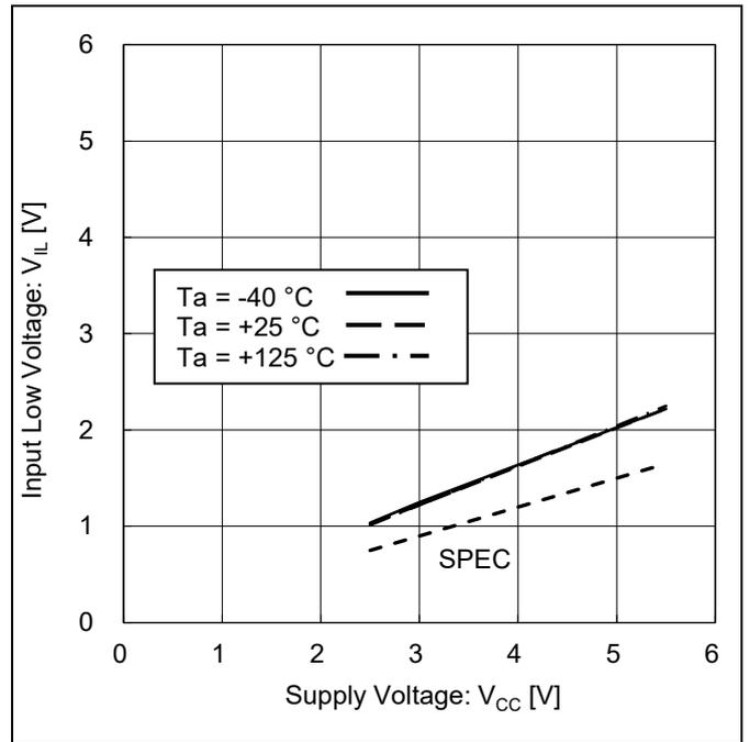
Figure 7. Input Low Voltage vs Supply Voltage
