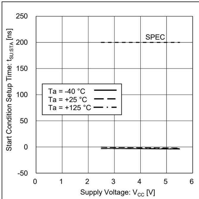
Figure 20. Start Condition Setup Time vs Supply Voltage
