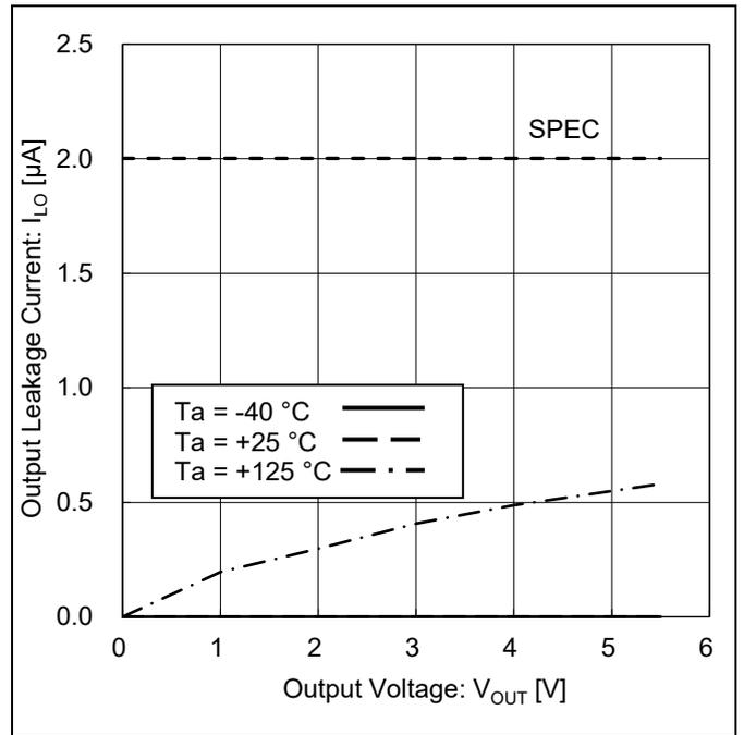
Figure 11. Output Leakage Current vs Output Voltage
