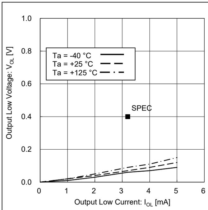
Figure 8. Output Low Voltage vs Output Low Current
