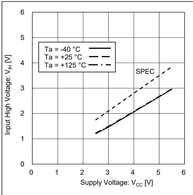
Figure 6. Input High Voltage vs Supply Voltage
