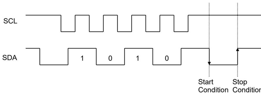
Figure 49. The Case of Cancel by Start, Stop Condition during Slave Address Input
