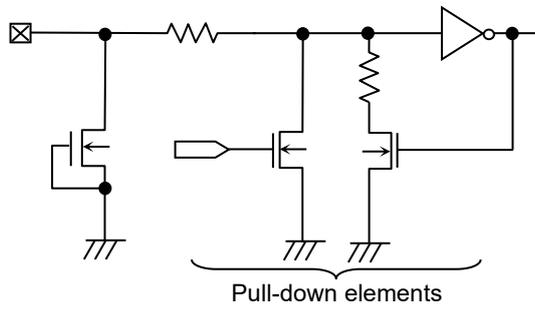
Figure 57. Input Pin Circuit Diagram (A1, A2, WP)
