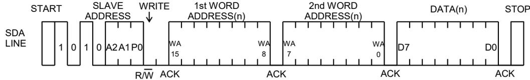
Figure 40. Byte Write
