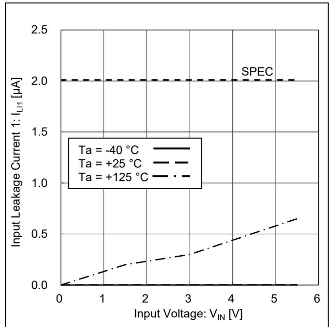
Figure 9. Input Leakage Current 1 vs Input Voltage
