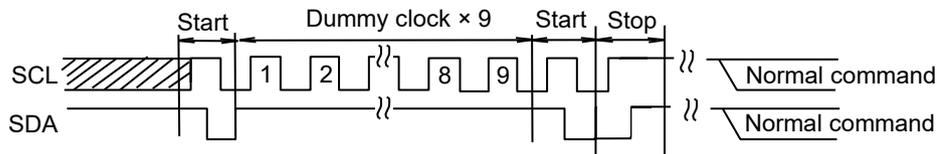
Figure 46. Input Timing of Software Reset
