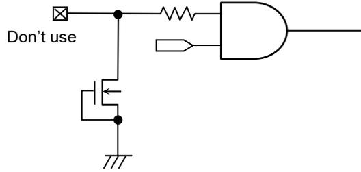
Figure 56. Input Pin Circuit Diagram (A0)
