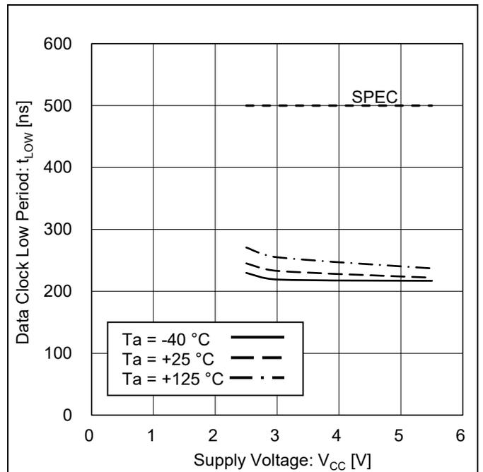
Figure 17. Data Clock Low Period vs Supply Voltage
