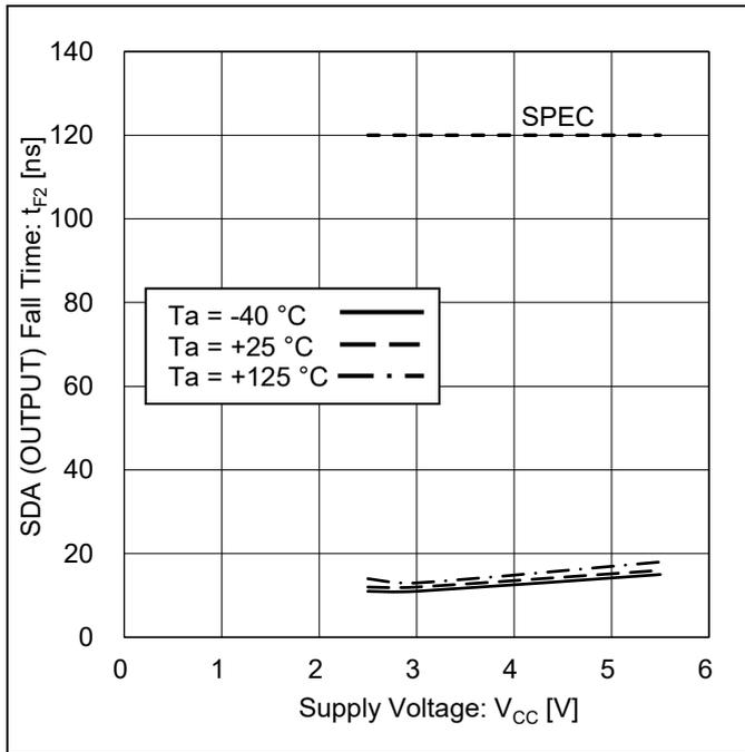
Figure 18. SDA (output) Fall Time vs Supply Voltage
