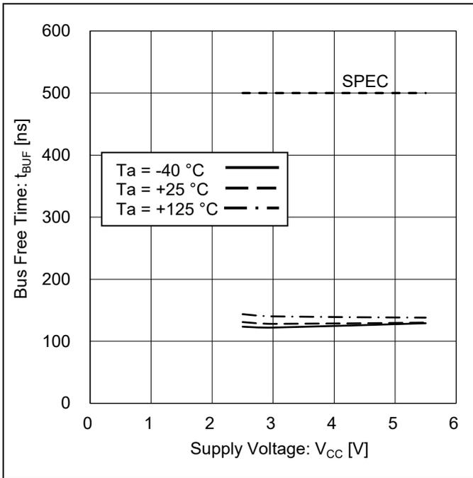
Figure 30. Bus Free Time vs Supply Voltage
