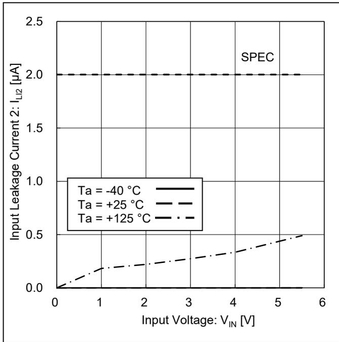
Figure 10. Input Leakage Current 2 vs Input Voltage
