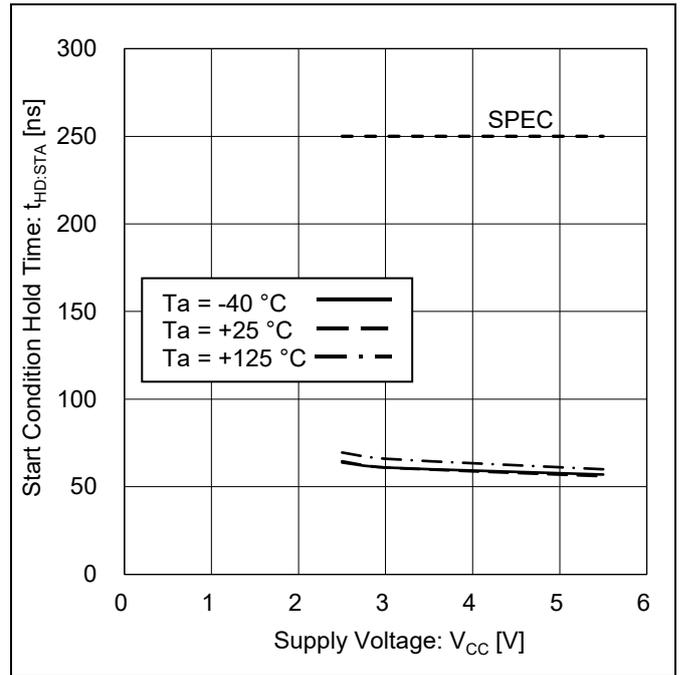
Figure 19. Start Condition Hold Time vs Supply Voltage
