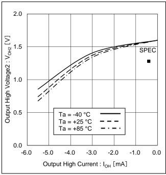
Figure 12. Output High Voltage2 vs Output High Current ( $V_{CC} = 1.6 \text{ V}$ )
