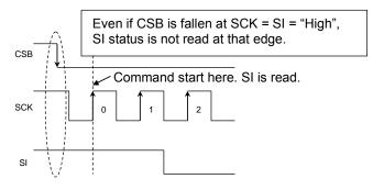
Figure 51. Operating Timing
