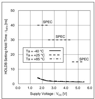
Figure 30. HOLDB Setting Hold Time vs Supply Voltage
