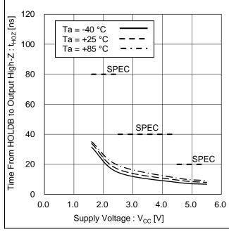
Figure 31. HOLDB Release Hold Time vs Supply Voltage
