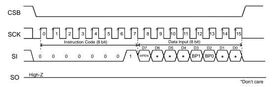
Figure 46. Write Status Register Command
