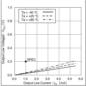
Figure 10. Output Low Voltage2 vs Output Low Current ( $V_{\text{CC}} = 1.6 \text{ V}$ )
