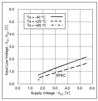
Figure 8. Input Low Voltage 1,2 vs Supply Voltage (CSB, SCK, SI, HOLDB, WPB)
