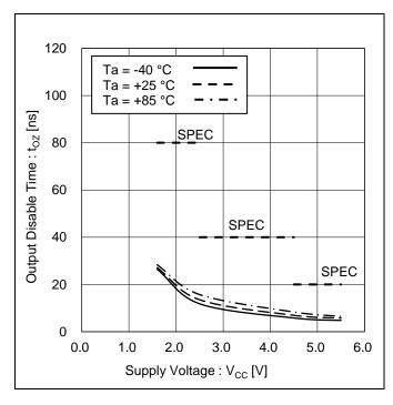
Figure 29. Output Disable Time vs Supply Voltage
