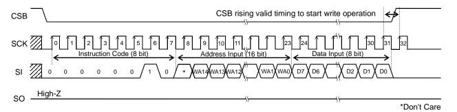
Figure 42. Write Command (Byte Write)
