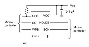
Figure 1. Typical Application Circuit
