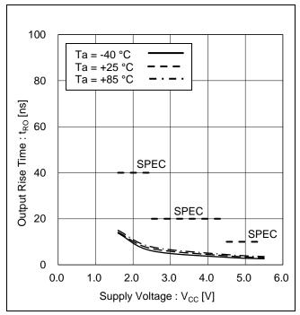
Figure 34. Output Rise Time vs Supply Voltage
