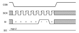
Figure 39. Write Enable Command
