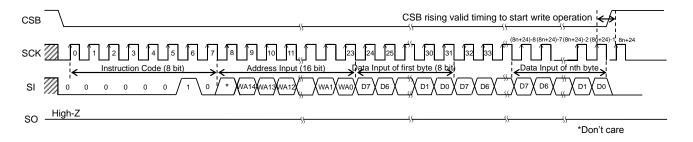
Figure 43. Write Command (Page Write)
