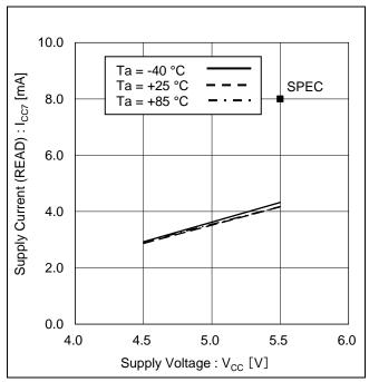
Figure 18. Supply Current (READ) vs Supply Voltage
