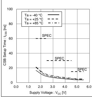
Figure 23. CSB High Time vs Supply Voltage
