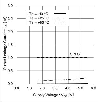
Figure 14. Output Leakage Current vs Supply Voltage (SO)
