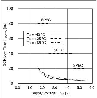
Figure 22. SCK Low Time vs Supply Voltage
