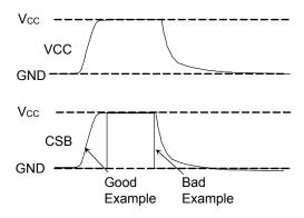
Figure 63. CSB Timing at power ON/OFF
