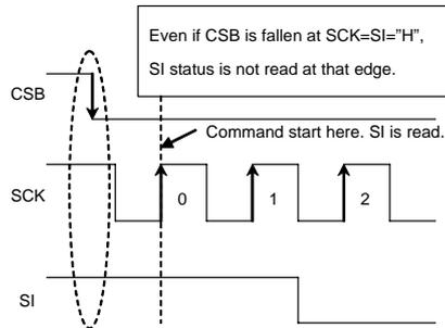
Figure 43. Operating timing
