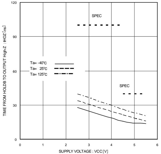
Figure 30. Time from HOLDB to Output High-Z tHOZ
