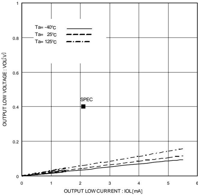
Figure 9. Output Low Voltage  $V_{OL}$ ,  $I_{OL}$
