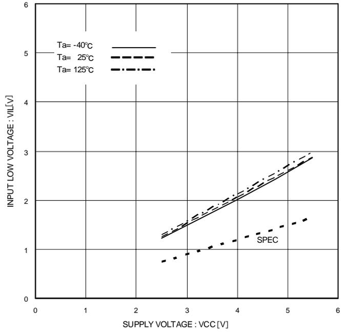
Figure 8. Input Low voltage  $V_{IL}$
