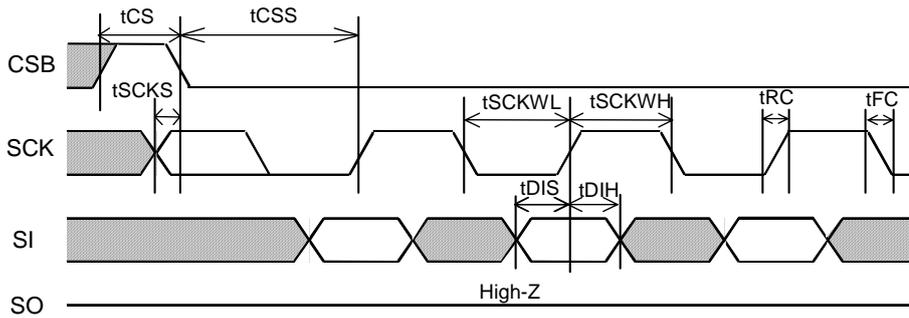
Figure 2. Input timing
