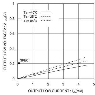
Figure 7. Output low voltage2 VoL2 (VCC=1.7V)
