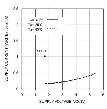
Figure 13. Supply current (WRITE) I<sub>CC1</sub>(WRITE, f<sub>SK</sub>=1MHz)
