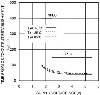
Figure 31. Time from CS to output establishment tsv
