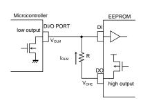
Conditions  $V_{ILE} \ge V_{OHE} - I_{OLM} \times R$ As this moment, VohE=VCC  $V_{ILE} \ge VCC - I_{OLM} \times R$
