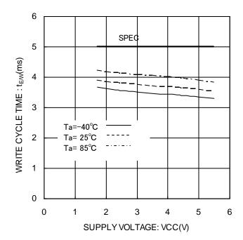
Figure 33. Write cycle time te/w
