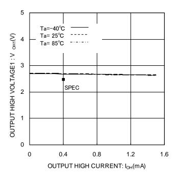
Figure 8. Output high voltage1 V<sub>OH1</sub>(VCC=2.7V)
