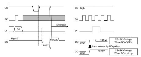
Figure 45. READY output timing at DO=OPEN
