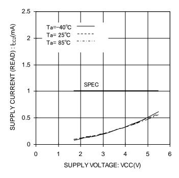
Figure 16. Supply current (READ)  $I_{CC2}(READ, f_{SK}=3MHz)$
