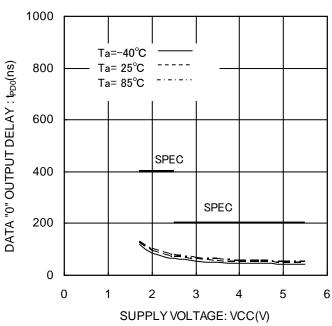
Figure 29. Data "0" output delay tPD0
