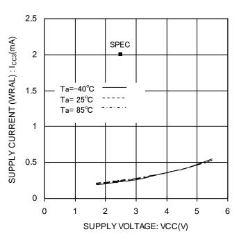
Figure 17. Supply current (WRAL) I<sub>CC3</sub>(WRAL,f<sub>SK</sub>=1MHz)
