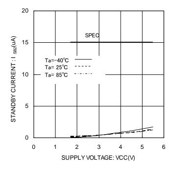
Figure 20. Standby current I<sub>SB2</sub>(CS=0V, ORG=0V)
