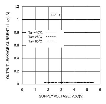
Figure 12. Output leakage current ILO(DO)
