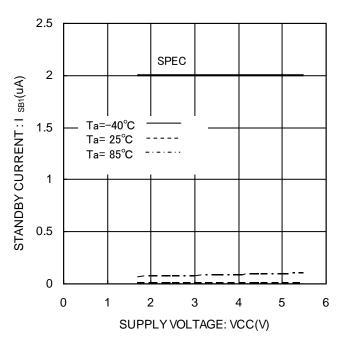
Figure 19. Standby current I<sub>SB1</sub>(CS=0V, ORG=VCC or OPEN)
