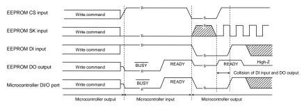
Figure 51. Collision timing at DI, DO direct connection
