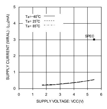
Figure 18. Supply current (WRAL) ICC3(WRAL,fsk=3MHz)
