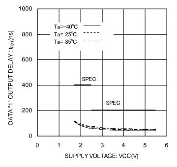
Figure 30. Data "1" output delay tPD1
