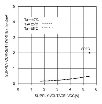
Figure 14. Supply current (WRITE) Icc1(WRITE,fsk=3MHz)
