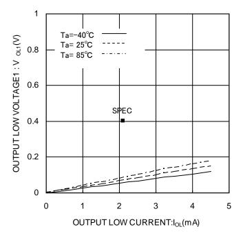
Figure 6. Output low voltage1 VoL1(VCC=2.7V)
