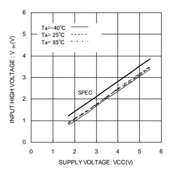
Figure 4. Input high voltage V<sub>IH</sub> (CS,SK,DI,ORG)
