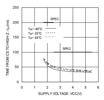
Figure 32. Time from CS to High-Z  $t_{DF}$
