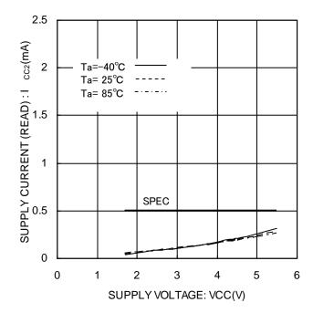
Figure 15. Supply current (READ) Icc2(READ,fsk=1MHz)
