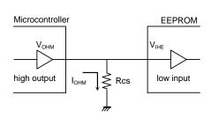
Figure 44. CS pull down resistance
