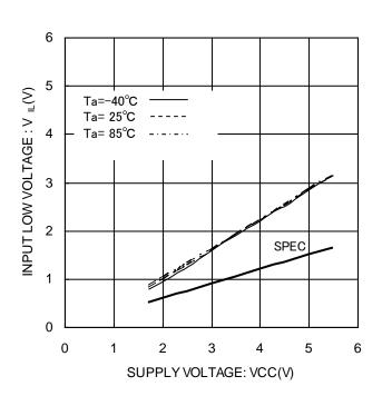
Figure 5. Input low voltage V<sub>IL</sub>(CS,SK,DI,ORG)
