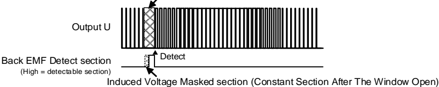
Figure 37. FG Mask Release Condition at Startup (FGALTIME setting count consecutively met): Output Signal Waveform When Induced Voltage Stability is Detected
