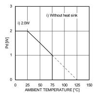
Fig.8 Thermal derating curve (BA6238A, HSIP10)
