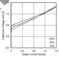
Fig.6 Output low voltage (BA6238A)
