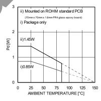
Fig.7 Thermal derating curve (BA6247FP-Y, HSOP25)
