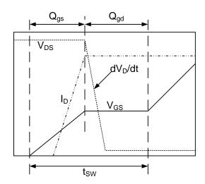
Figure 14. Gate Charge Transfer Characteristics
