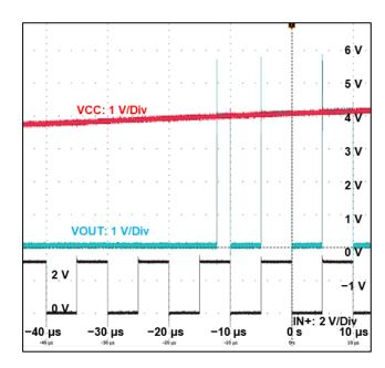
Figure 8. Startup Time (0  $\Omega$  as Routh and Routl, 220 pF load)
