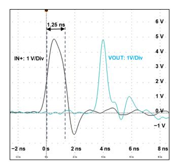
Figure 9. Shutdown Time (0  $\Omega$  as Routh and Routl, 220 pF load)
