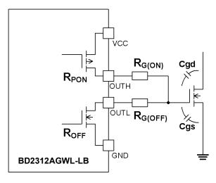
Figure 13. Gate Driver Equivalent Circuit
