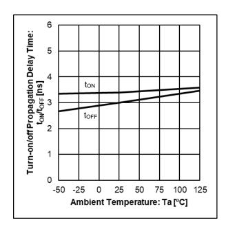
Figure 7. Turn-on/off Propagation Delay Time vs Ambient Temperature (VCC = 5 V, 0  $\Omega$  as R<sub>OUTH</sub> and R<sub>OUTL</sub>, 100 pF load)
