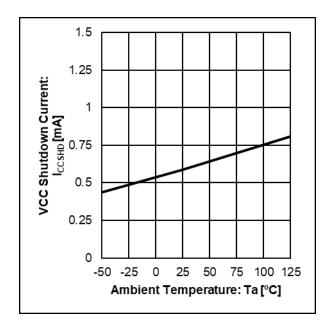
Figure 4. VCC Shutdown Current vs Ambient Temperature  $(VCC = 5 \text{ V}, \text{V}_{\text{IN+}} = \text{V}_{\text{EN}} = 0 \text{ V})$
