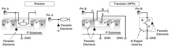
Figure 16. Example of Monolithic IC Structure
