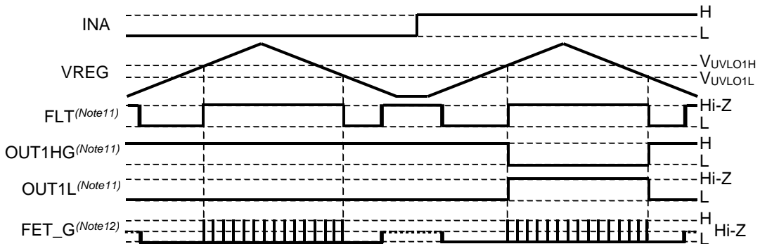
Figure 76. VREG UVLO Function Operation Timing Chart
