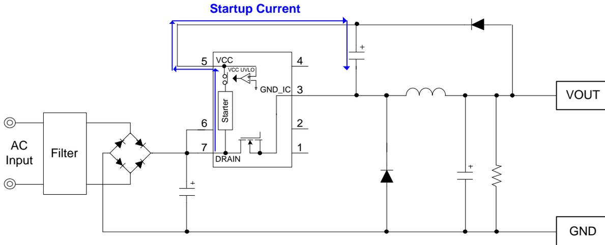
Figure 5. Startup Circuit
