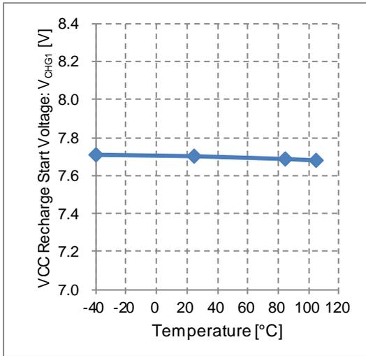
Figure 24. VCC Recharge Start Voltage vs Temperature (BM2P101X-Z, BM2P121X-Z)
