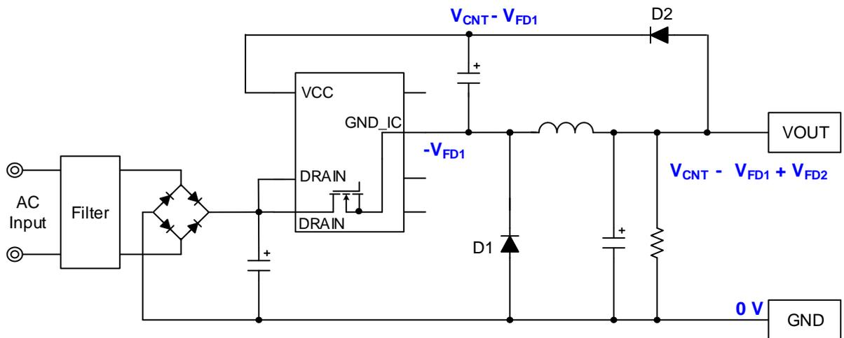
Figure 8. Back Converter Circuit (MOSFET = OFF)
