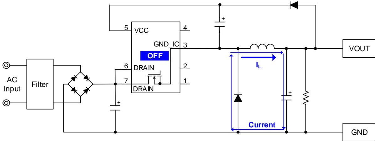
Figure 2. Back Converter Operation (MOSFET = OFF)
