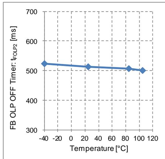
Figure 31. FB OLP OFF Timer vs Temperature
