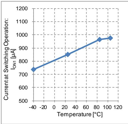
Figure 16. Current at Switching Operation vs Temperature
