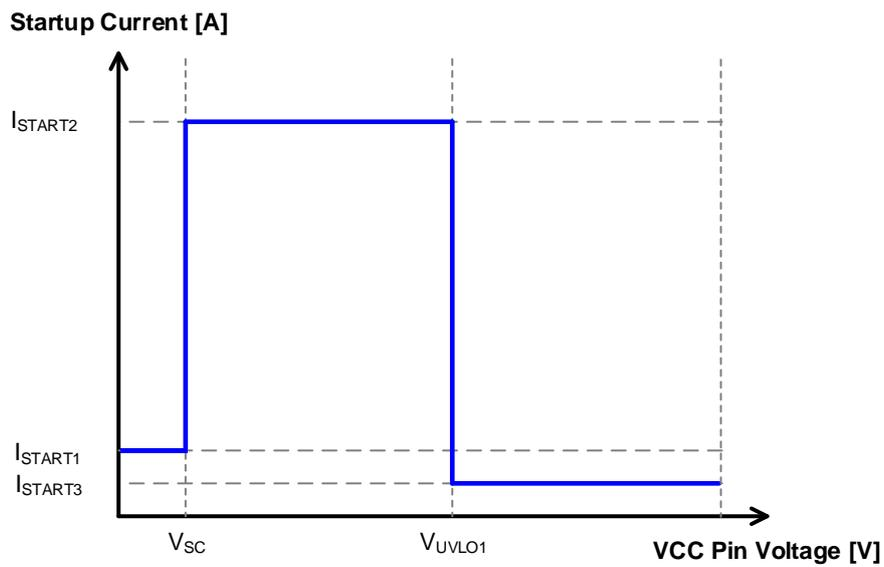
Figure 6. Startup Current vs VCC Pin Voltage
