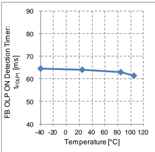
Figure 30. FB OLP ON Detection Timer vs Temperature
