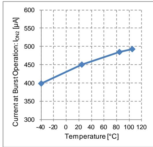
Figure 17. Current at Burst Operation vs Temperature
