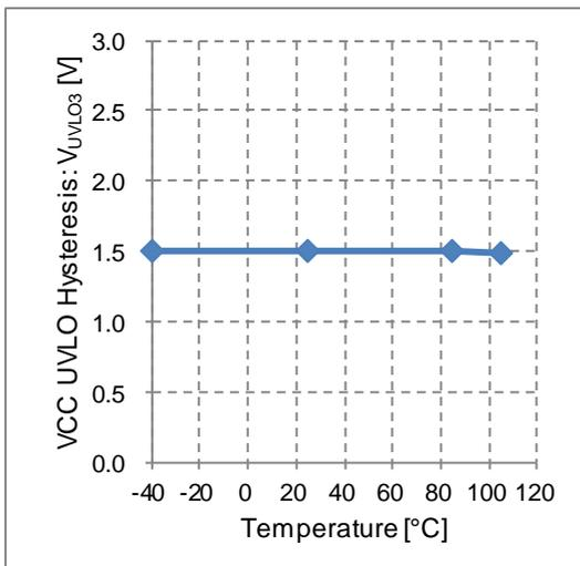
Figure 22. VCC UVLO Hysteresis vs Temperature (BM2P101X-Z, BM2P121X-Z)
