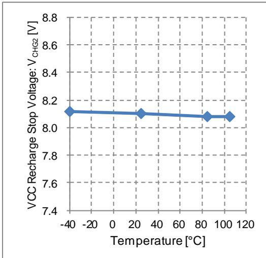
Figure 26. VCC Recharge Stop Voltage vs Temperature (BM2P101X-Z, BM2P121X-Z)
