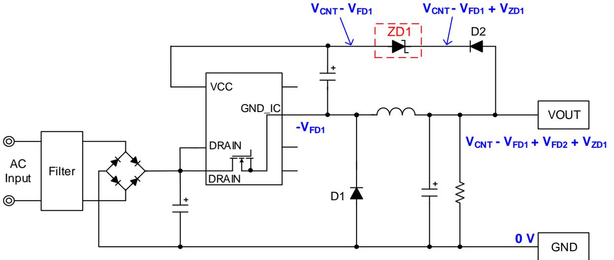
Figure 10. Back Converter Output Dispersion Circuit (MOSFET = OFF)
