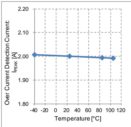
Figure 32. Over Current Detection Current vs Temperature
