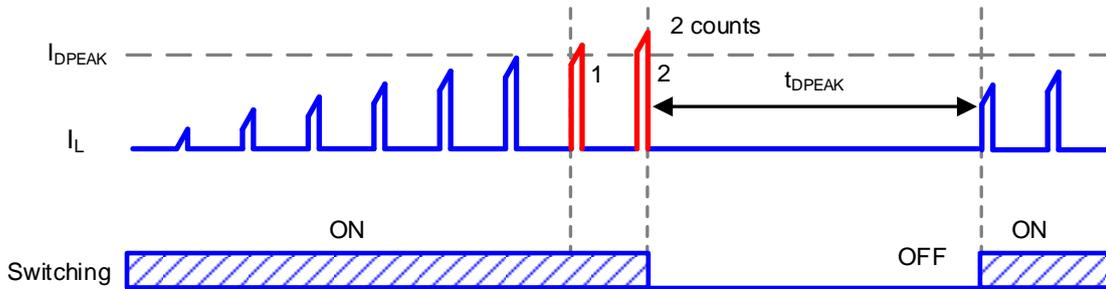
Figure 12. Dynamic Over Current Limiter
