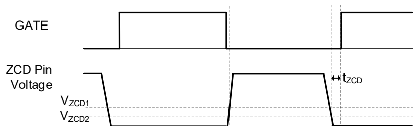
Figure 11. Zero Current Detection Operation
