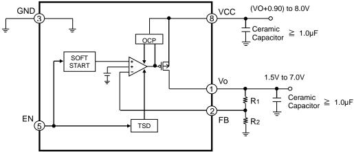
Fig.1 Block Diagram
