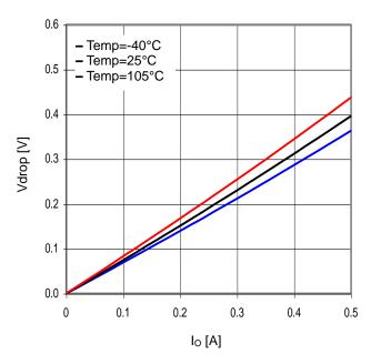
Fig. 34 Minimum dropout Voltage 1 (Vcc=4.5V)
