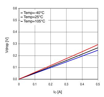
Fig. 36 Minimum dropout Voltage 3  $(V_{CC}=8.0V)$
