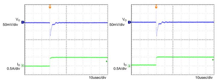
Fig.3 Transient Response (0→0.5A) Co=1µF, Ta=-40°C
