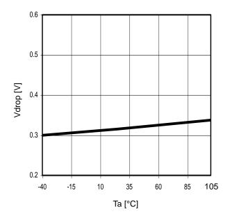
Fig. 33 Ta-Vdrop (Vcc=6V, Io=0.5A)
