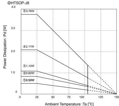
Measure condition: mounted on a ROHM board, and IC
