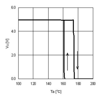
Fig. 28 TSD (I<sub>O</sub>=0mA)
