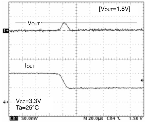
Figure 17. Transient Response ( $I_o=2A$  to  $1A$ ,  $10\mu s$ )
