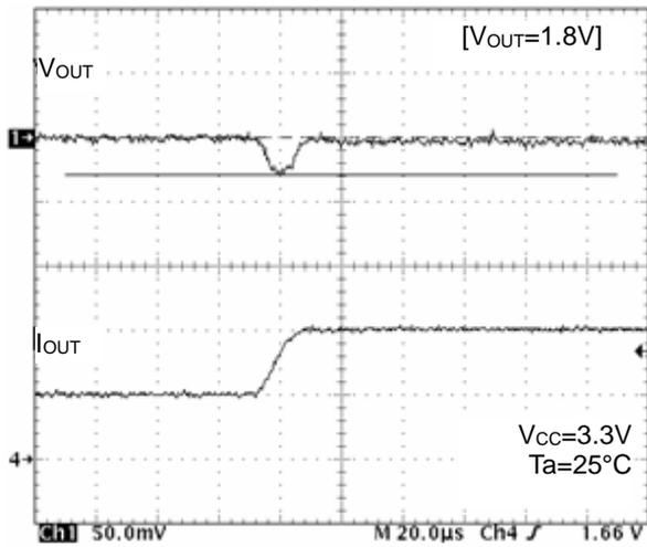
Figure 16. Transient Response ( $I_o=1A$  to  $2A$ ,  $10\mu s$ )
