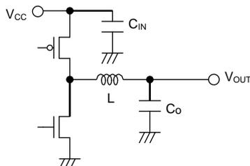
Figure 28. Input Capacitor
