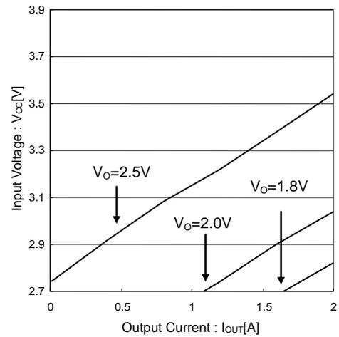
Figure 33. Minimum Input Voltage in each Output Voltage
