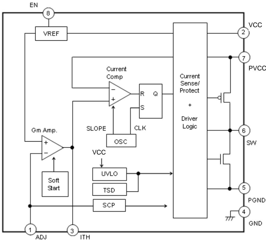
Figure 3. Block Diagram
