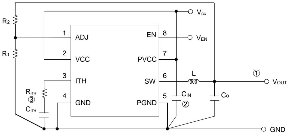
Figure 34. Layout Diagram
