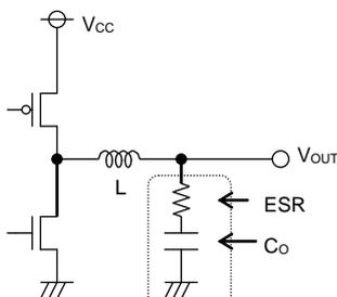
Figure 27. Output Capacitor
