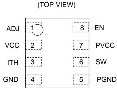
Figure 2. Pin Configuration
