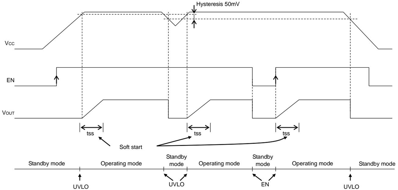
Figure 20. Soft Start, Shutdown, UVLO Timing Chart
