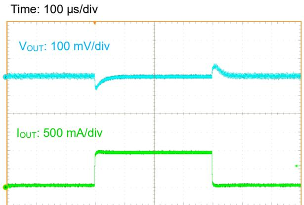
Figure 57. Load Transient Response ( $I_{OUT} = 0.1\text{ A}$  to  $1.0\text{ A}$ )
