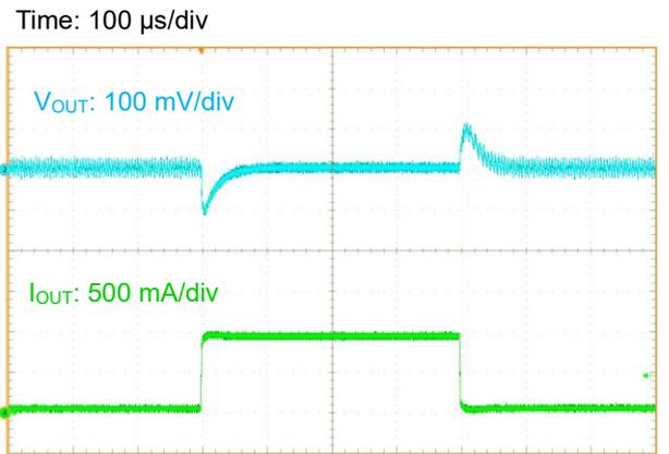
Figure 52. Load Transient Response ( $I_{OUT} = 0.1\text{ A to } 1.0\text{ A}$ )
