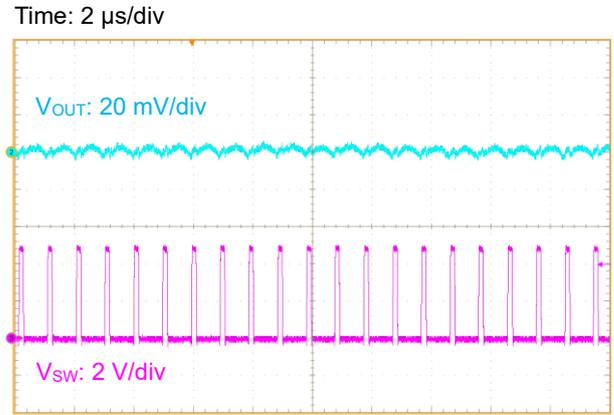
Figure 65. Output Ripple Voltage ( $I_{OUT} = 3.0\text{ A}$ )
