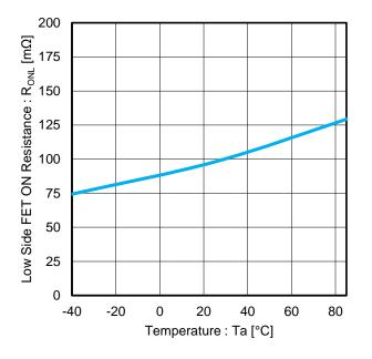
Figure 13. Low Side FET ON Resistance vs Temperature
