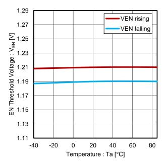
Figure 4. EN Threshold Voltage vs Temperature
