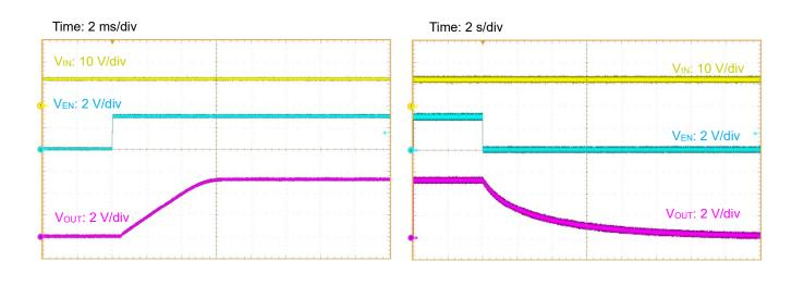
Figure 17. Start-up at No load: V<sub>EN</sub> = 0 V to 3 V (V<sub>IN</sub> = 12 V, V<sub>OUT</sub> = 5 V)
