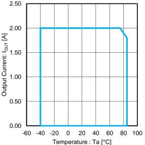
Figure 21. Output Current vs Temperature<sup>(Note 1)</sup> Operating Range: Tj < 150 °C ( $V_{IN}$  = 12 V,  $V_{OUT}$  = 3.3 V)
