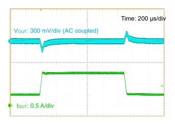
Figure 47. Load Transient Response (V\_{IN} = 24 V, I\_{OUT} = 0.5 A to 1.5 A)
