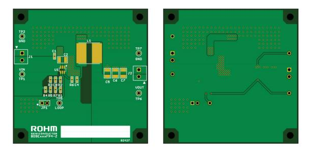
Figure 53. Example of PCB Layout (Silkscreen Overlay)
