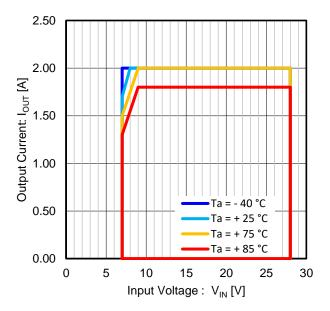
Figure 25. Output Current vs Input Voltage<sup>(Note 1)</sup> (Note 2) Operating Range: Tj < 150 °C (V<sub>OUT</sub> = 5.0 V)
