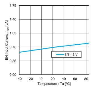
Figure 5. EN Input Current vs Temperature
