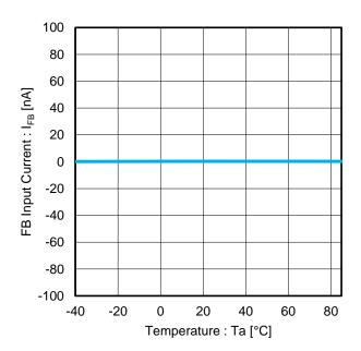
Figure 8. FB Input Current vs Temperature
