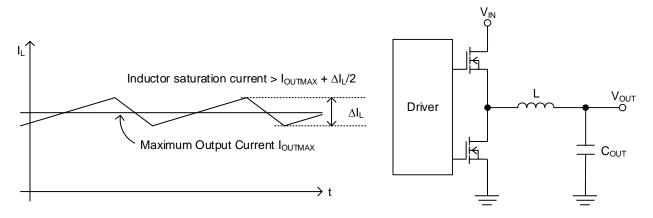
Figure 48. Waveform of Inductor Current
