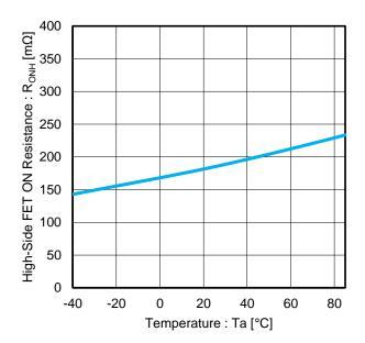
Figure 12. High Side FET ON Resistance vs Temperature
