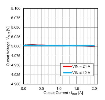
Figure 15. Output Voltage vs Output Current
