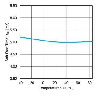
Figure 9. Soft Start Time vs Temperature
