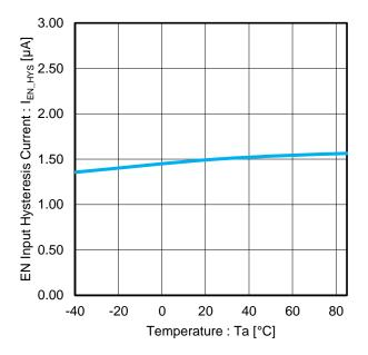
Figure 6. EN Input Hysteresis Current vs Temperature
