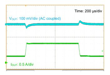
Figure 37. Load Transient Response  $(V_{IN} = 12 \text{ V}, I_{OUT} = 0.5 \text{ A to } 1.5 \text{ A})$
