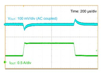
Figure 42. Load Transient Response  $(V_{IN} = 12 \text{ V}, I_{OUT} = 0.5 \text{ A to } 1.5 \text{ A})$
