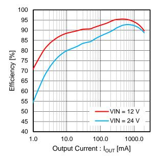
Figure 39. Efficiency vs Output Current
