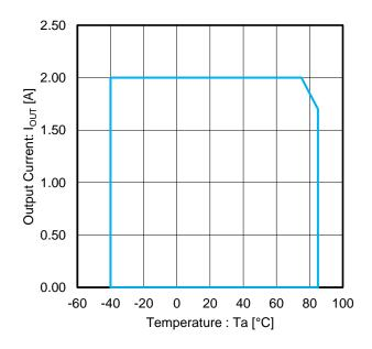
Figure 23. Output Current vs Temperature<sup>(Note 1)</sup> Operating Range: Tj < 150 °C ( $V_{IN}$  = 24 V,  $V_{OUT}$  = 12 V)
