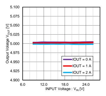
Figure 16. Output Voltage vs Input Voltage
