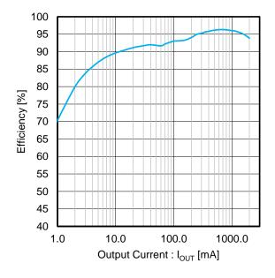
Figure 44. Efficiency vs Output Current
