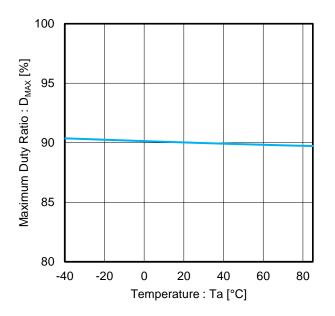
Figure 11. Maximum Duty Ratio vs Temperature
