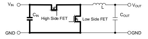
Figure 51-c. Difference of Current and Critical Area in Layout
