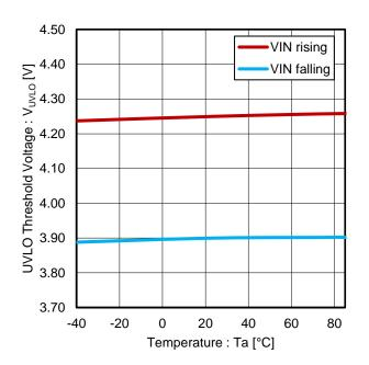
Figure 3. UVLO Threshold Voltage vs Temperature
