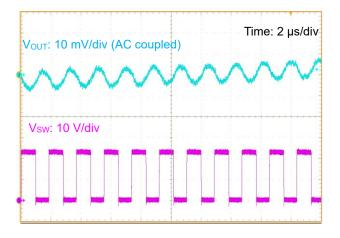
Figure 45. Output Ripple Voltage (VIN = 24 V, IOUT = 2 A)
