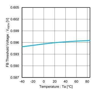
Figure 7. FB Threshold Voltage vs Temperature
