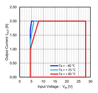
Figure 24. Output Current vs Input Voltage<sup>(Note 1)</sup> (Note 2) Operating Range: Tj < 150 °C ( $V_{OUT} = 3.3 V$ )
