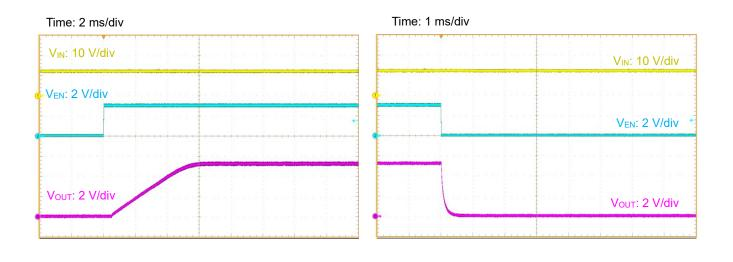
Figure 19. Start-up at R<sub>LOAD</sub> = 2.5  $\Omega$ : V<sub>EN</sub> = 0 V to 3 V (V<sub>IN</sub> = 12 V, V<sub>OUT</sub> = 5 V)
