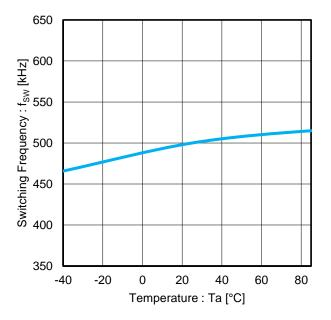
Figure 10. Switching Frequency vs Temperature
