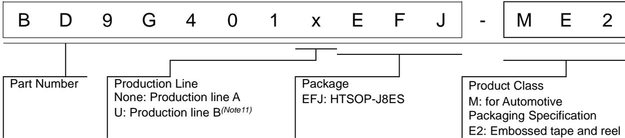
(Note11) For the purpose of improving production efficiency, this product has multi-line configuration. Electric characteristics noted in this datasheet does not differ between the 2 lines. Production line B is recommended for new product.
