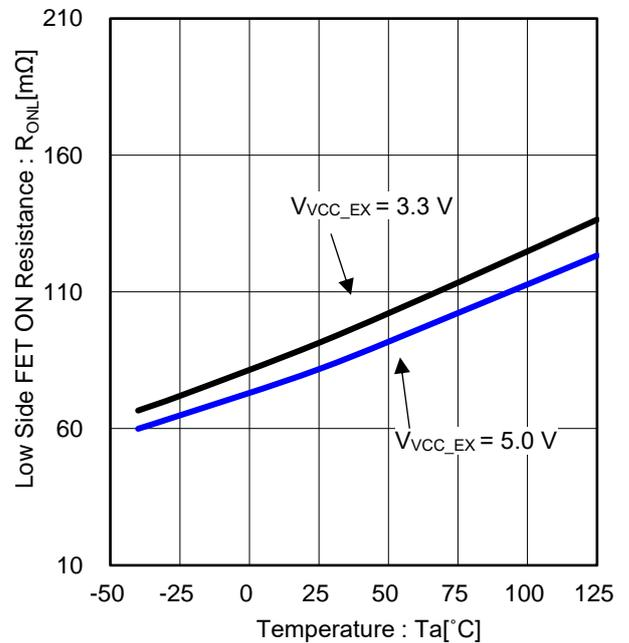
Figure 16. Low Side FET ON Resistance vs Temperature
