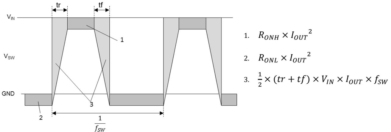
Figure 70. SW Waveform
