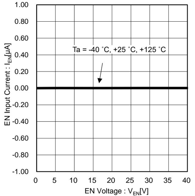
Figure 10. EN Input Current vs EN Voltage
