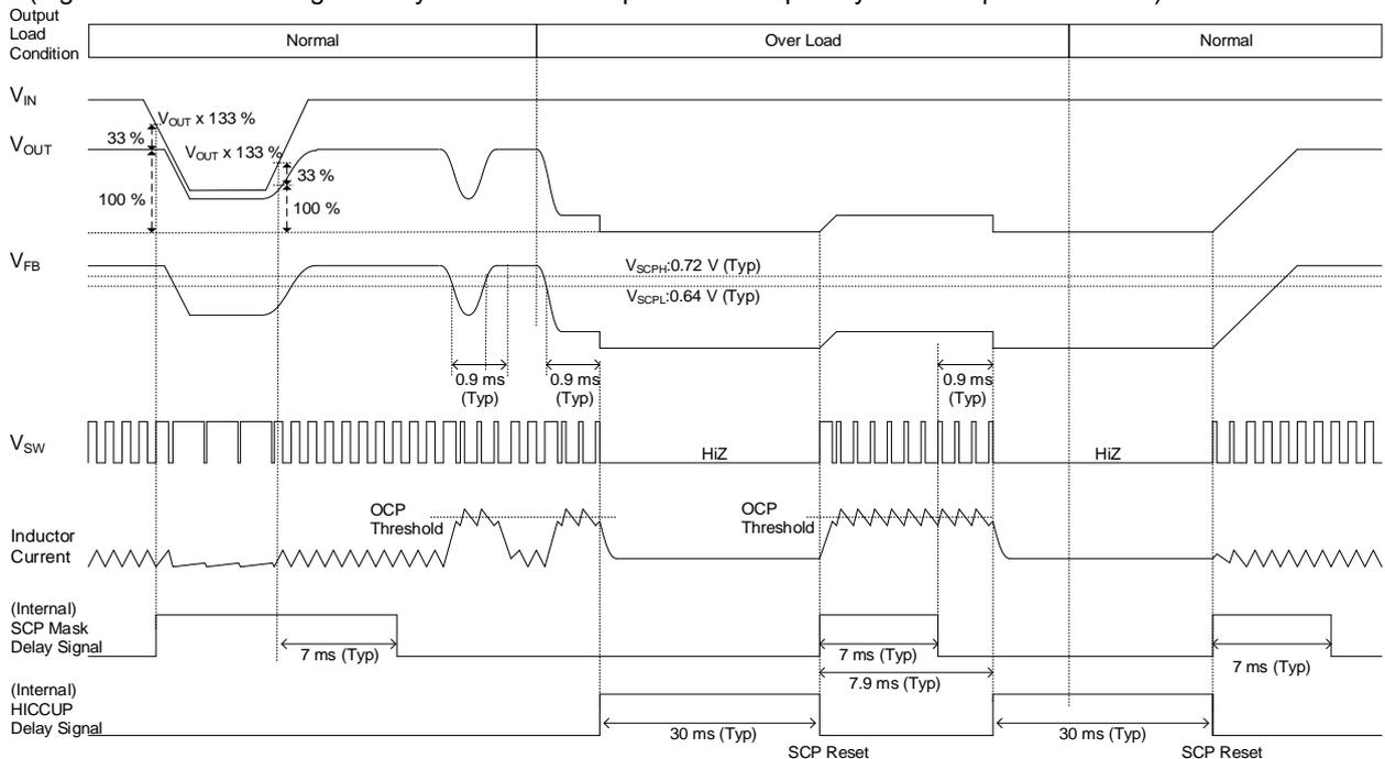
Figure 32. Short Circuit Protection (SCP) Timing Chart
