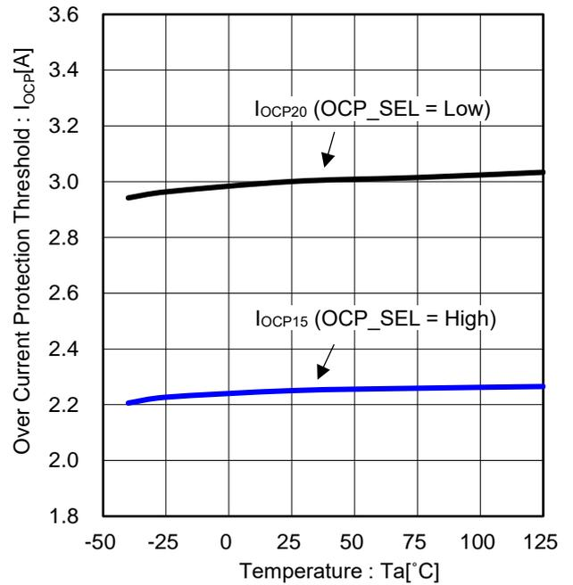
Figure 14. Over Current Protection Threshold vs Temperature
