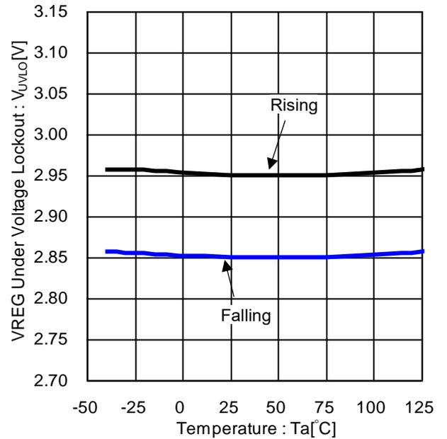
Figure 8. VREG Under Voltage Lockout vs Temperature
