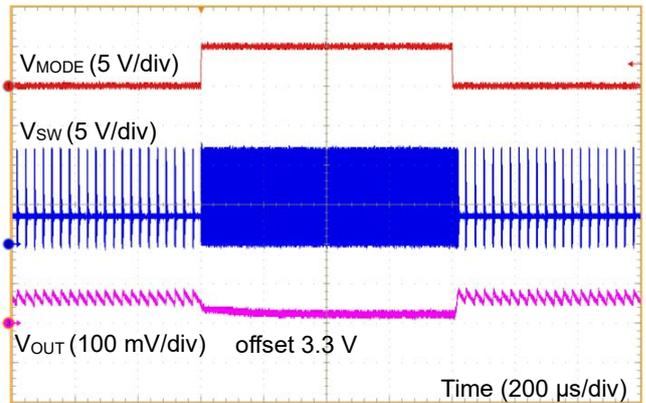
Figure 44. MODE ON/OFF Response (VIN = 12 V, IOUT = 50 mA)
