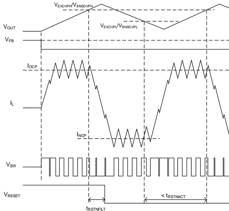
Figure 36. VCC\_EX/VOUT\_SNS OVP Timing Chart
