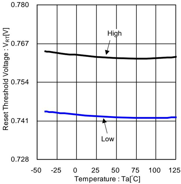
Figure 17. Reset Threshold Voltage vs Temperature
