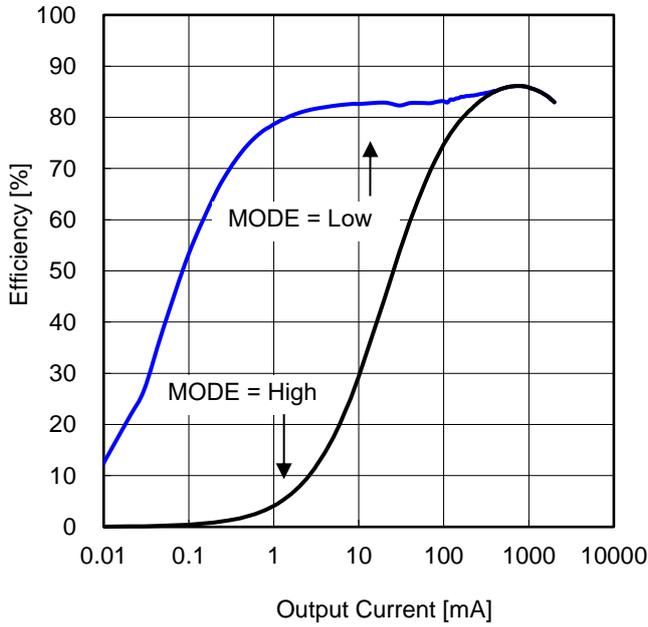
Figure 41. Efficiency vs Output Current (VIN = 12 V)
