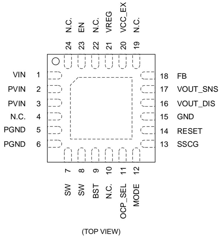
Figure 3. Pin Configuration
