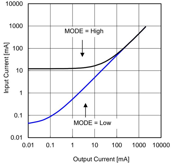
Figure 55. Input Current vs Output Current (VIN = 12 V)
