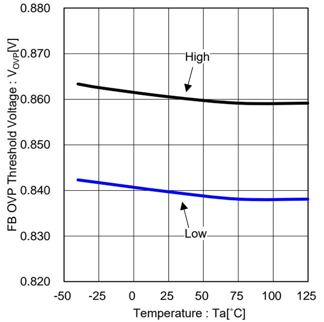
Figure 18. FB OVP Threshold Voltage vs Temperature
