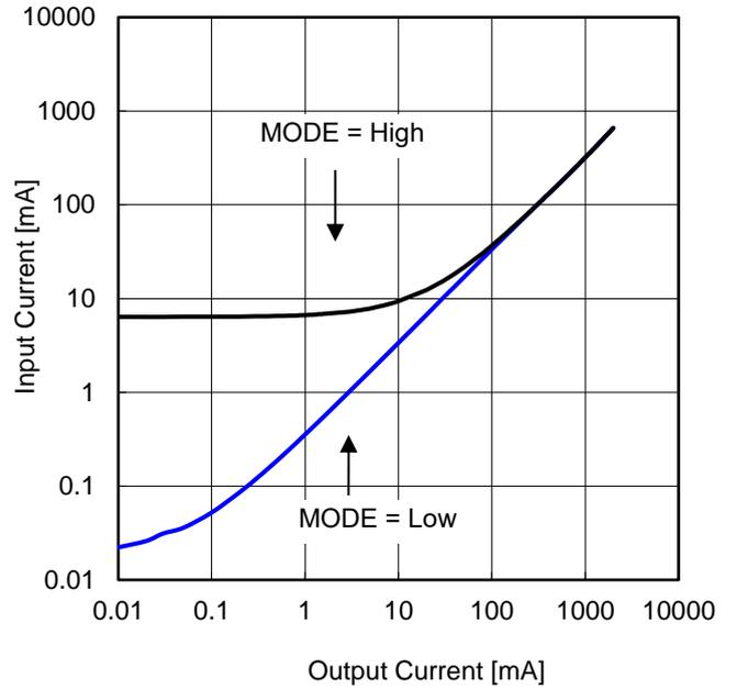
Figure 42. Input Current vs Output Current (VIN = 12 V)
