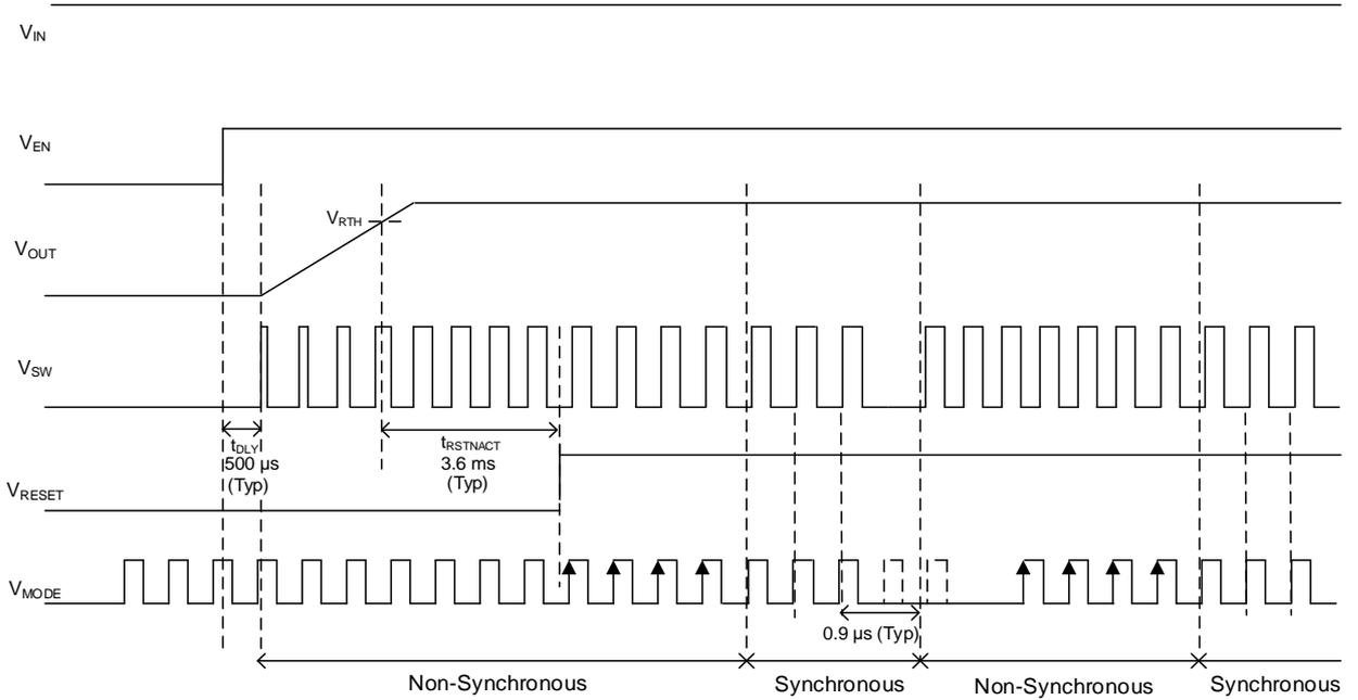
Figure 26. External Synchronization Function
