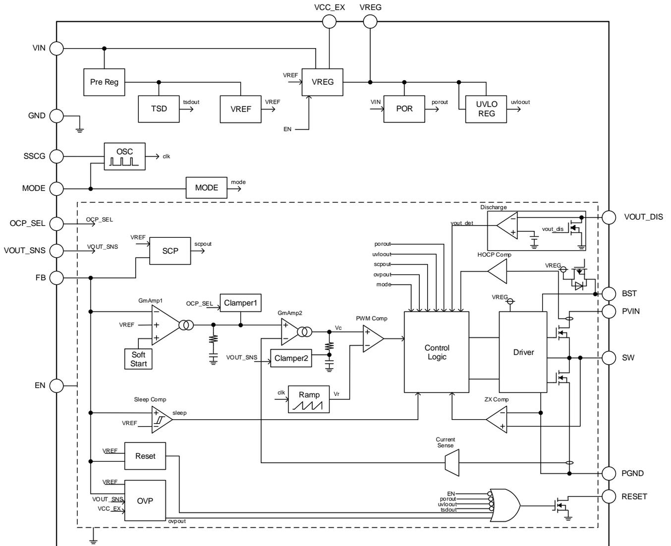
Figure 4. Block Diagram
