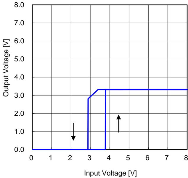
Figure 49. Output Voltage vs Input Voltage 1
