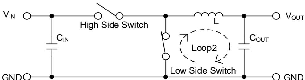
Figure 67 (b). Current Path when High Side Switch = OFF, Low Side Switch = ON
