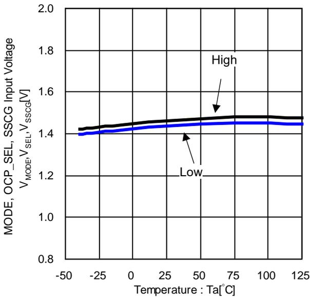
Figure 11. MODE, OCP\_SEL, SSCG Input Voltage vs Temperature
