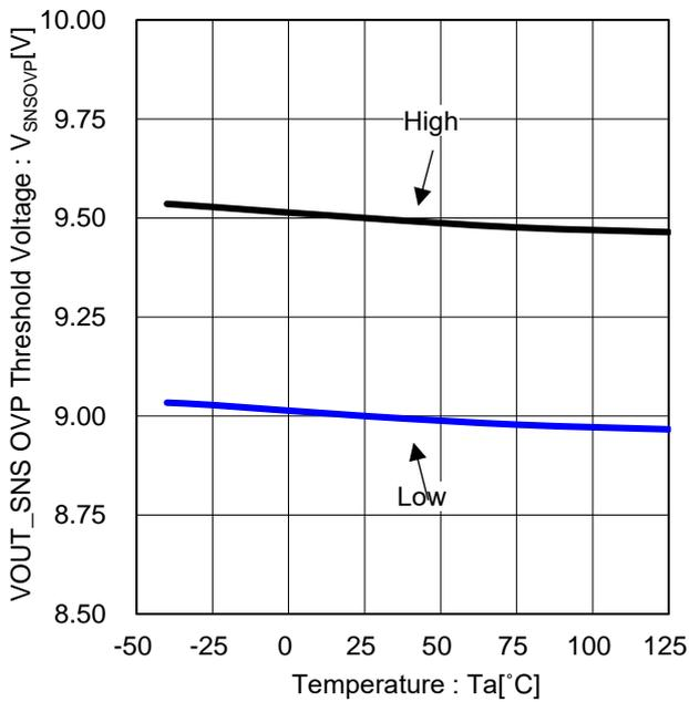
Figure 19. VOUT\_SNS OVP Threshold Voltage vs Temperature
