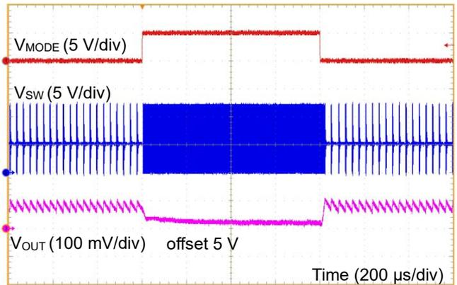
Figure 57. MODE ON/OFF Response (VIN = 12 V, IOUT = 50 mA)
