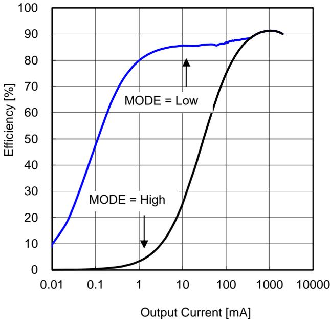
Figure 54. Efficiency vs Output Current (VIN = 12 V)
