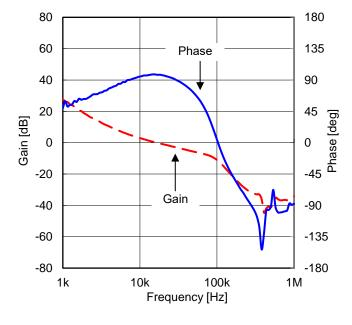
Figure 78. Frequency Characteristic (V<sub>IN</sub> = 12 V, I<sub>OUT</sub> = 1.0 A)
