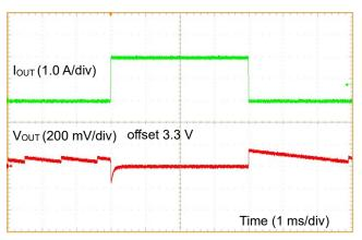
Figure 67. Load Response 1  $(V_{IN} = 12 \text{ V}, V_{MODE} = 5 \text{ V}, I_{OUT} = 0 \text{ A to } 2 \text{ A})$
