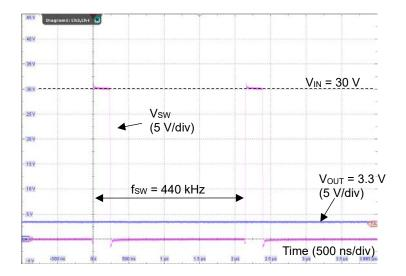
Figure 29. Switching Waveform ( $V_{IN} = 30 \text{ V}$ ,  $V_{OUT} = 3.3 \text{ V}$ ,  $I_{OUT} = 1.0 \text{ A}$ ,  $f_{SW} = 440 \text{ kHz}$ )
