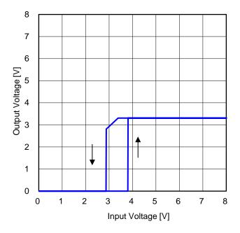
Figure 71. Output Voltage vs Input Voltage 1  $(R_{LOAD} = 165 \Omega)$
