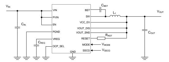
Figure 1. Application Circuit with Discharge Function (BD9P236EFV-C, BD9P256EFV-C)
