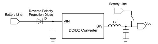
Figure 46. VOUT shorted to Battery Line
