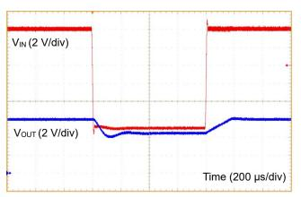
Figure 56. Line Response 1 ( $V_{IN}$  = 16 V to 8 V,  $I_{OUT}$  = 2 A)
