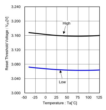
Figure 24. Reset Threshold Voltage vs Temperature (BD9P236EFV-C)
