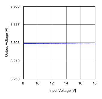
Figure 73. Line Regulation (I<sub>OUT</sub> = 2 A)
