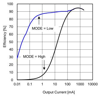
Figure 76. Efficiency vs Output Current  $(V_{IN} = 12 \text{ V})$
