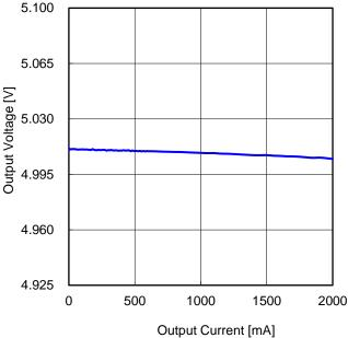
Figure 87. Load Regulation (V<sub>IN</sub> = 12 V)
