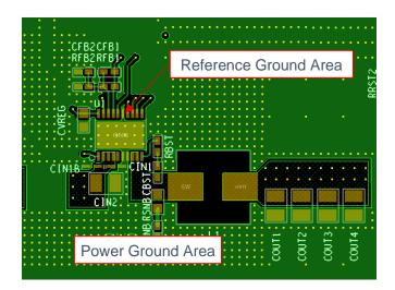
Figure 90. Recommended Board Layout Example (for BD9P206EFV-C)
