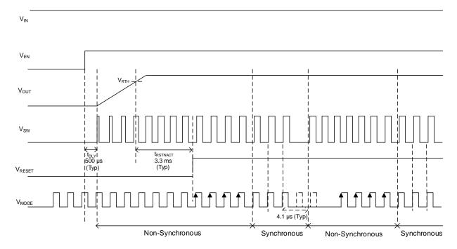
Figure 35. External Synchronization Function
