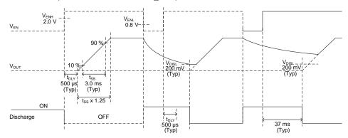
Figure 33. Enable ON/OFF Timing Chart
