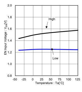
Figure 15. EN Input Voltage vs Temperature
