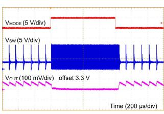
Figure 66. MODE ON/OFF Response (V<sub>IN</sub> = 12 V, I<sub>OUT</sub> = 50 mA)
