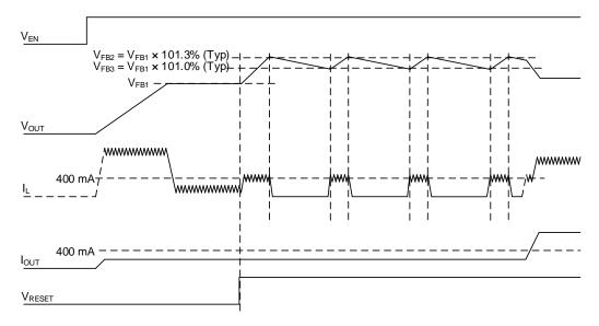
Figure 32. Timing Chart in Light Load Mode after Detecting RESET High (OCP SEL = L)
