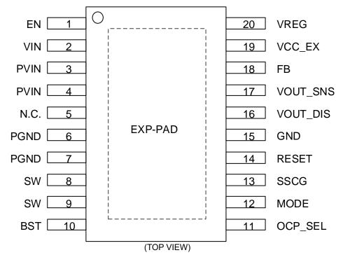
Figure 6. Pin Configuration (BD9P206EFV-C)
