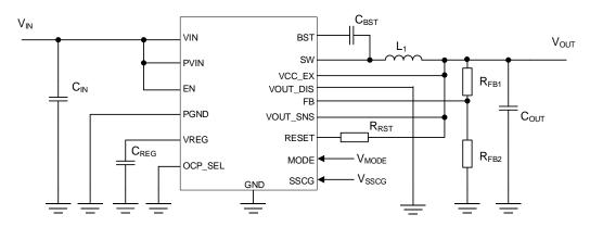
Figure 4. Application Circuit without Discharge Function (BD9P206EFV-C)
