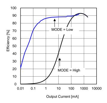
Figure 63. Efficiency vs Output Current (V<sub>IN</sub> = 12 V)
