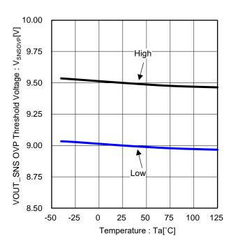
Figure 27. VOUT\_SNS OVP Threshold Voltage vs Temperature (BD9P206EFV-C)
