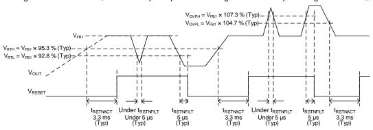
Figure 34. Reset Timing Chart (BD9P206EFV-C)
