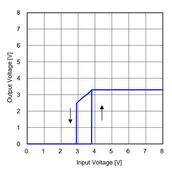
Figure 72. Output Voltage vs Input Voltage 2  $(R_{LOAD} = 1.65 \Omega)$
