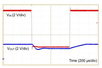
Figure 82. Line Response 1 ( $V_{IN}$  = 16 V to 8 V,  $I_{OUT}$  = 2 A)
