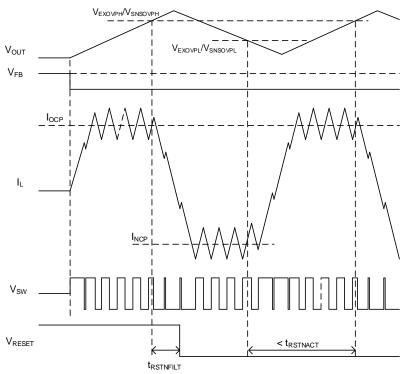
Figure 45. VCC\_EX/VOUT\_SNS OVP Timing Chart
