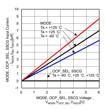
Figure 18. MODE, OCP\_SEL, SSCG Input Current vs MODE, OCP\_SEL, SSCG Voltage
