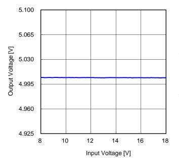
Figure 86. Line Regulation (I<sub>OUT</sub> = 2 A)
