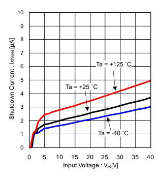
Figure 9. Shutdown Current vs Input Voltage
