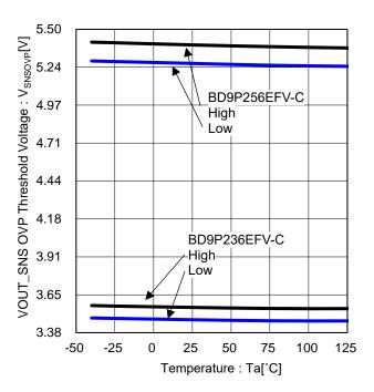
Figure 28. VOUT\_SNS OVP Threshold Voltage vs Temperature (BD9P236EFV-C/BD9P256EFV-C)
