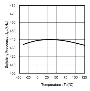
Figure 19. Switching Frequency vs Temperature
