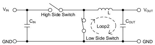
Figure 89 (b). Current Path when High Side Switch = OFF, Low Side Switch = ON
