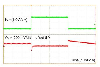
Figure 80. Load Response 1 ( $V_{IN}$  = 12 V,  $V_{MODE}$  = 5 V,  $I_{OUT}$  = 0 A to 2 A)
