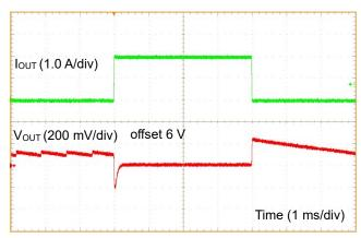
Figure 54. Load Response 1 ( $V_{IN}$  = 12 V,  $V_{MODE}$  = 5 V,  $I_{OUT}$  = 0 A to 2 A)
