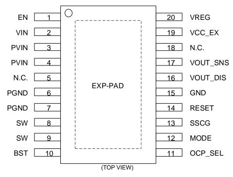
Figure 5. Pin Configuration (BD9P236EFV-C, BD9P256EFV-C)
