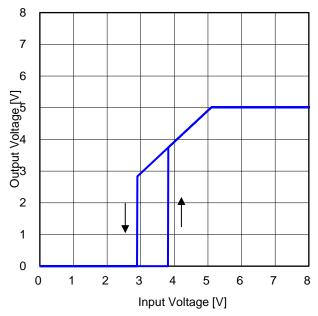
Figure 84. Output Voltage vs Input Voltage 1  $(R_{LOAD} = 250 \Omega)$
