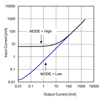
Figure 77. Input Current vs Output Current (V<sub>IN</sub> = 12 V)
