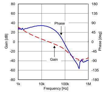
Figure 65. Frequency Characteristic ( $V_{IN} = 12 \text{ V}, I_{OUT} = 1.0 \text{ A}$ )
