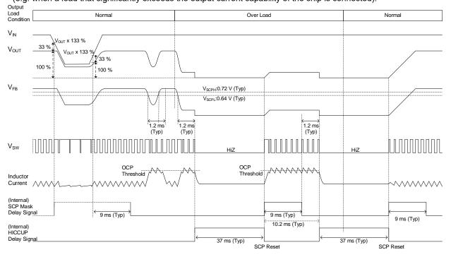
Figure 41. Short Circuit Protection (SCP) Timing Chart (BD9P206EFV-C)
