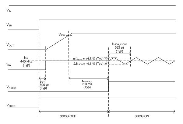
Figure 37. Spread Spectrum Function
