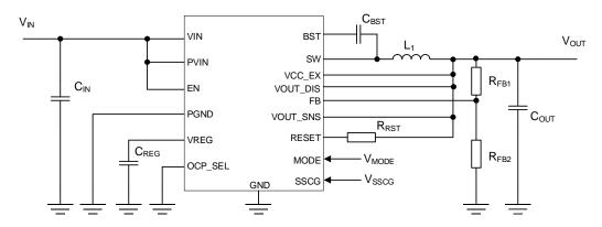
Figure 3. Application Circuit with Discharge Function (BD9P206EFV-C)
