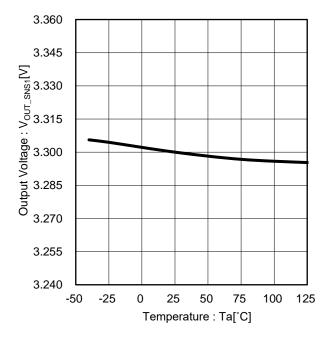
Figure 11. Output Voltage vs Temperature (BD9P236EFV-C)
