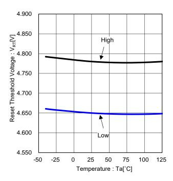
Figure 25. Reset Threshold Voltage vs Temperature (BD9P256EFV-C)
