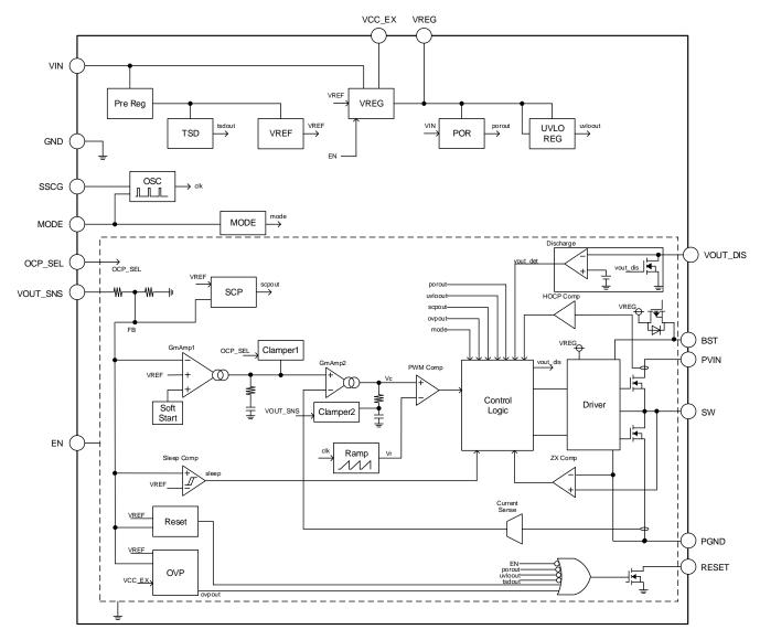
Figure 8. Block Diagram (BD9P236EFV-C, BD9P256EFV-C)
