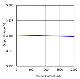
Figure 74. Load Regulation (V<sub>IN</sub> = 12 V)
