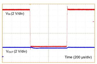
Figure 69. Line Response 1  $(V_{IN} = 16 \text{ V to } 8 \text{ V}, I_{OUT} = 2 \text{ A})$
