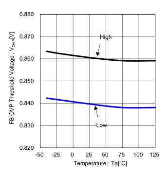
Figure 26. FB OVP Threshold Voltage vs Temperature (BD9P206EFV-C)
