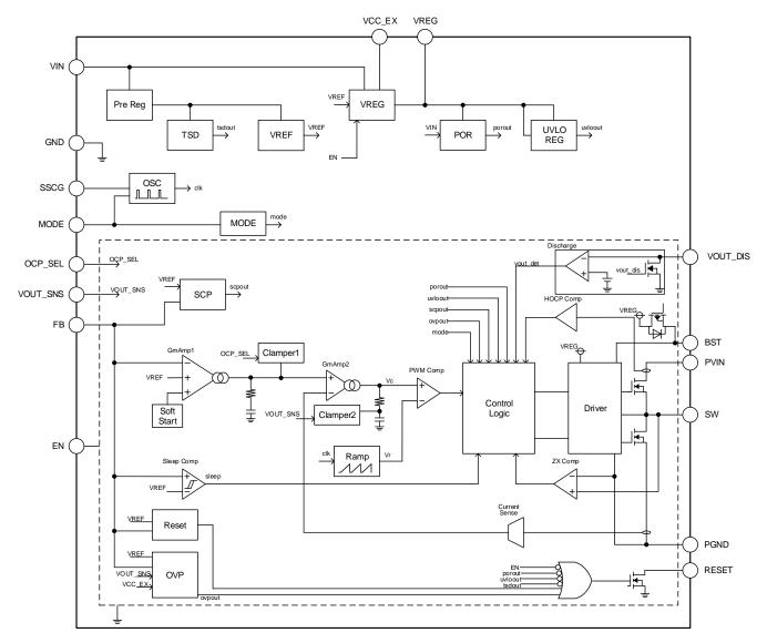
Figure 7. Block Diagram (BD9P206EFV-C)
