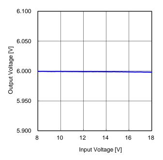
Figure 60. Line Regulation (I<sub>OUT</sub> = 2 A)
