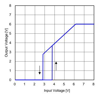
Figure 58. Output Voltage vs Input Voltage 1  $(R_{LOAD} = 300 \Omega)$
