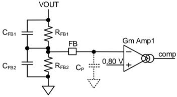
Figure 48. Setting for Output Setting Resistor
