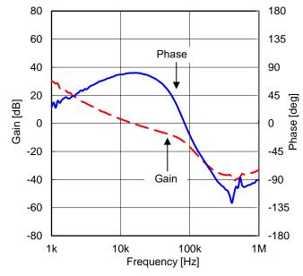
Figure 52. Frequency Characteristic ( $V_{IN}$  = 12 V,  $I_{OUT}$  = 1.0 A)
