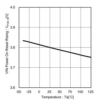
Figure 14. VREG Under Voltage Lockout vs Temperature
