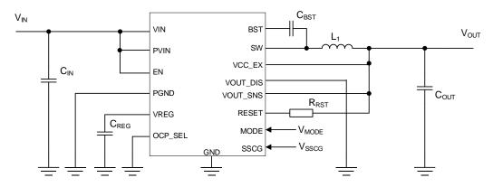
Figure 2. Application Circuit without Discharge Function (BD9P236EFV-C, BD9P256EFV-C)
