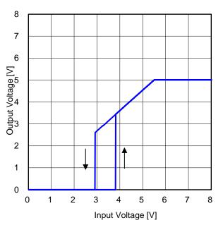
Figure 85. Output Voltage vs Input Voltage 2  $(R_{LOAD} = 2.5 \Omega)$
