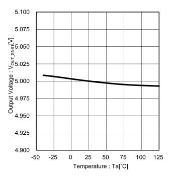
Figure 12. Output Voltage vs Temperature (BD9P256EFV-C)
