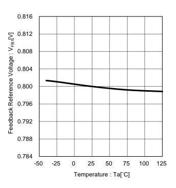
Figure 10. Feedback Reference Voltage vs Temperature (BD9P206EFV-C)
