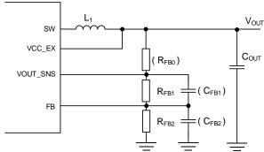
Figure 91. The resistor for measuring the frequency characteristic of the feedback
