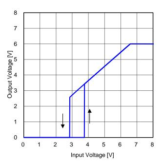
Figure 59. Output Voltage vs Input Voltage 2  $(R_{LOAD} = 3 \Omega)$
