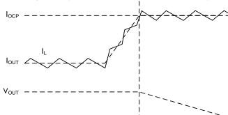
Figure 40. Over Current Protection
