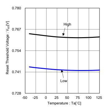
Figure 23. Reset Threshold Voltage vs Temperature (BD9P206EFV-C)
