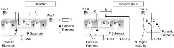
Figure 93. Example of Monolithic IC Structure
