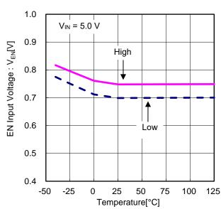
Figure 13. UVLO Voltage vs Temperature
