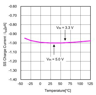
Figure 5. Soft Start Time vs Temperature
