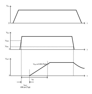
Figure 19. Enable ON/OFF Timing Chart
