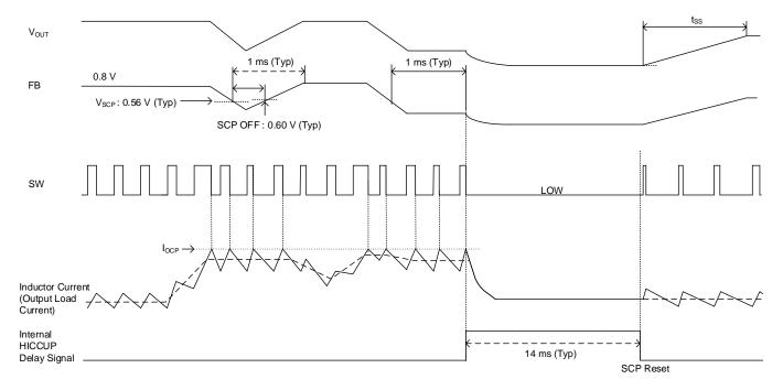
Figure 22. Short Circuit Protection (SCP) Timing Chart
