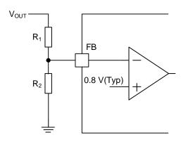
Figure 26. Feedback Resistor Circuit
