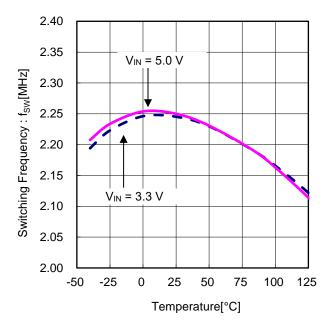
Figure 3. Switching Frequency vs Temperature
