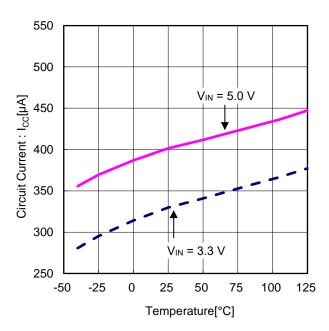
Figure 2. Circuit Current vs Temperature
