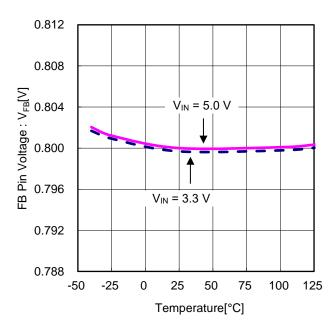
Figure 4. FB Pin Voltage vs Temperature
