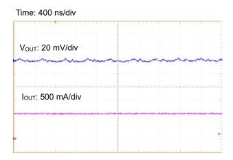
Figure 54. Output Ripple Voltage (I<sub>OUT</sub> = 1 A)
