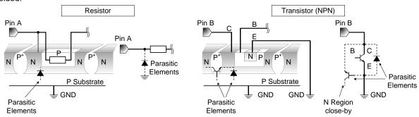
Figure 60. Example of Monolithic IC Structure
