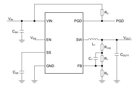
Figure 40. Measurement Circuit 3
