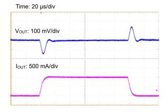
Figure 53. Load Transient Response (Iouт = 0 A ↔ 1 A)
