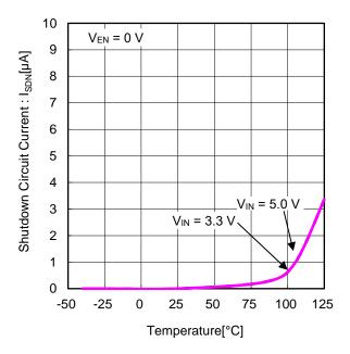
Figure 1. Shutdown Circuit Current vs Temperature
