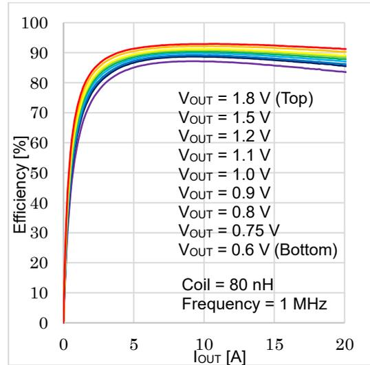
Figure 18. Efficiency vs  $I_{OUT}$  (w/o DCR loss)(VIN = 5 V, Ta = 25 °C)
