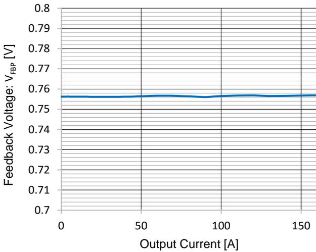
Figure 5. Feedback Voltage (8phase) vs Output Current ( $V_{IN} = 5.0\text{ V}$ ,  $T_a = 25\text{ }^\circ\text{C}$ )
