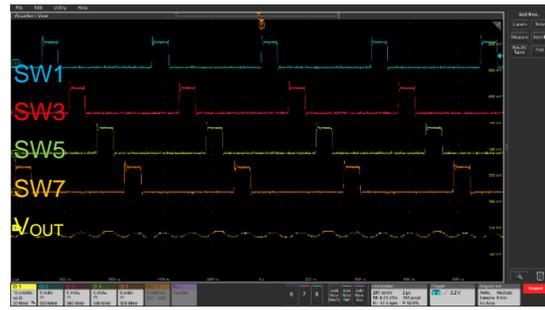
Figure 13. BD9634x series SW Pin and Ripple Voltage(8phase)1/2 (VIN = 5.0 V, Ta = 25 °C)
