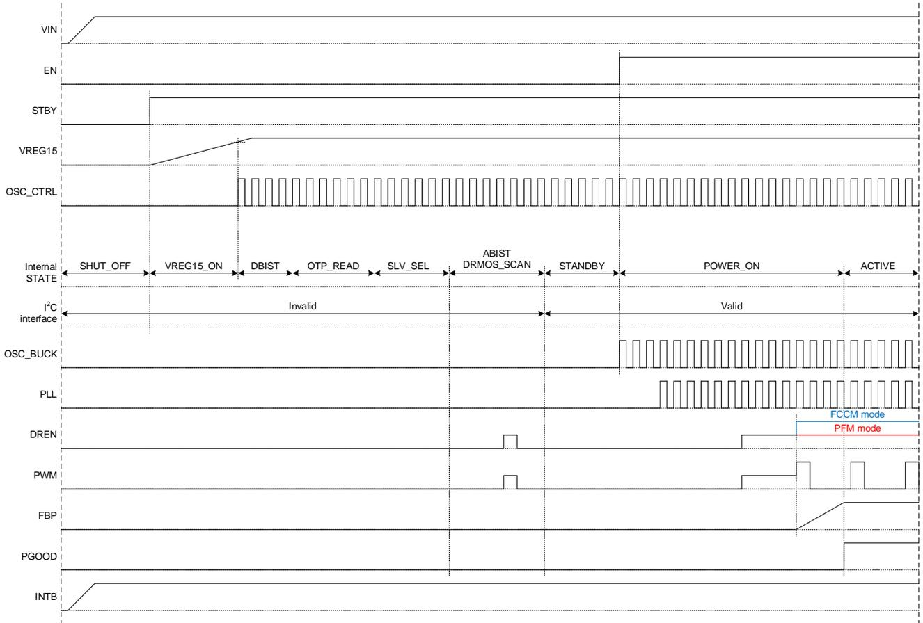
Figure 21. STBY ON, EN ON Sequence Timing Chart
