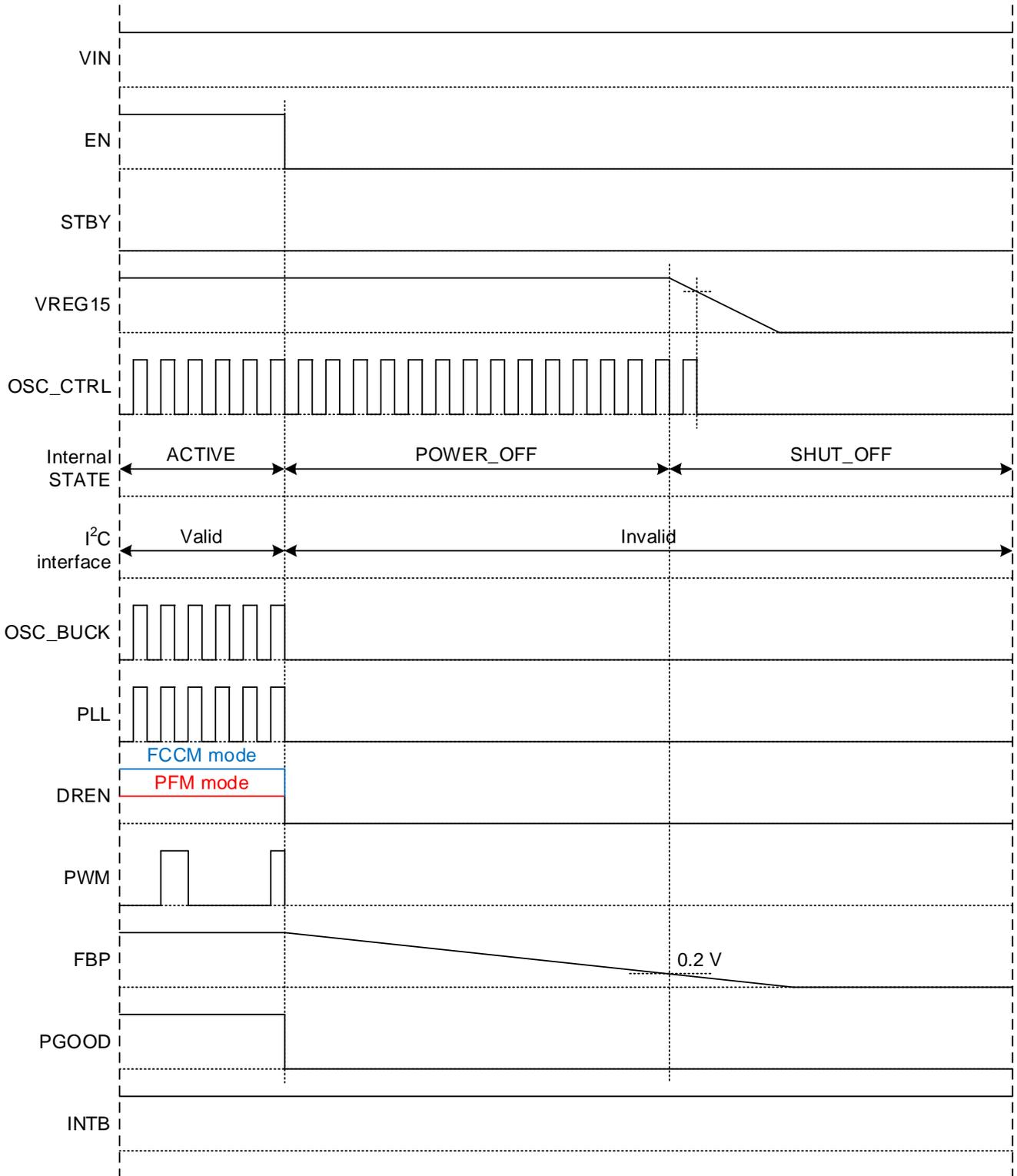
Figure 23. EN OFF (STBY OFF) Sequence Timing Chart
