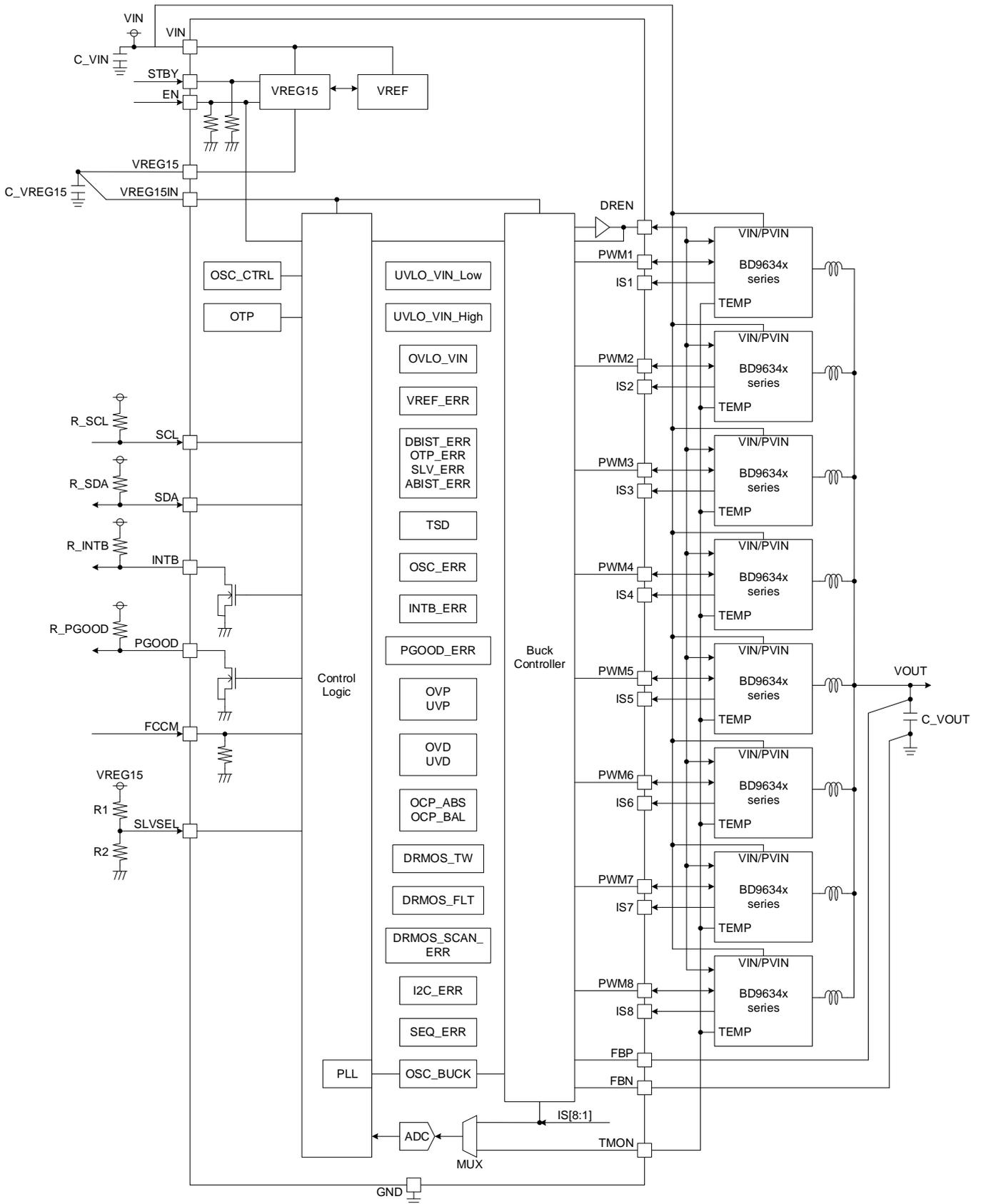
Figure 2. Block Diagram
