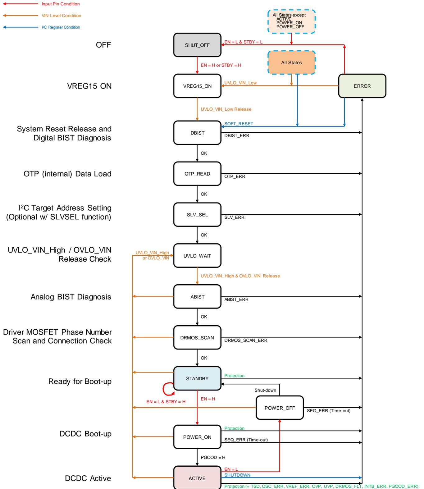
Figure 19. State Transition Diagram
