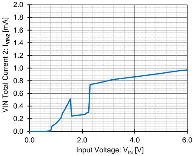
Figure 3. VIN Total Current 2 vs Input Voltage 1 ( $T_a = 25\text{ }^\circ\text{C}$ )
