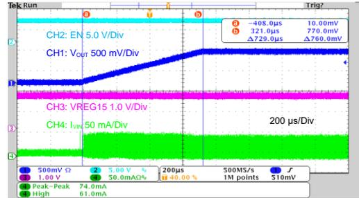
Figure 10. Soft Start Waveform(Zoom Up)
