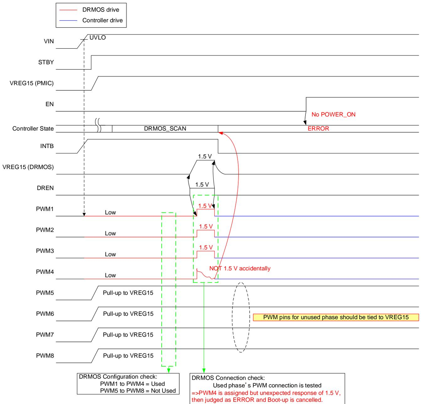
Figure 35. Driver MOSFET Phase Number Scan Example (Error case 2)
