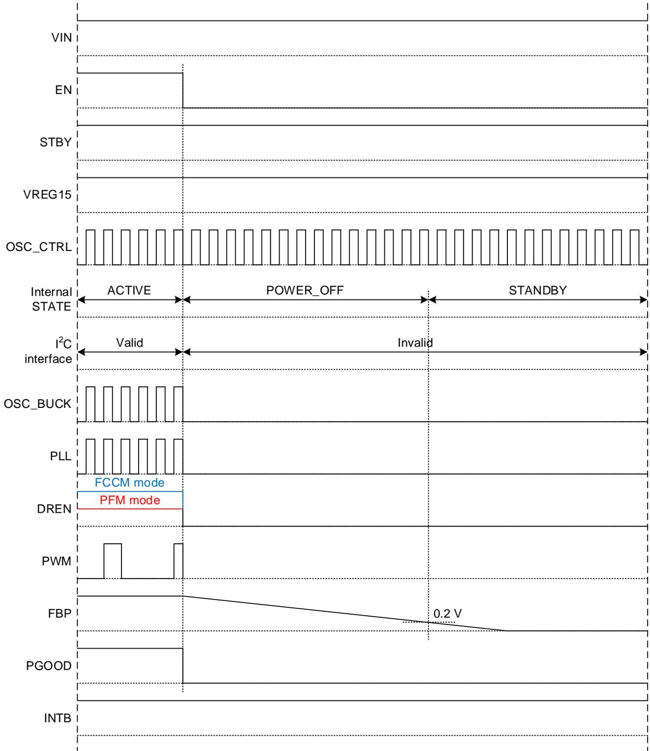
Figure 22. EN OFF (STBY ON) Sequence Timing Chart
