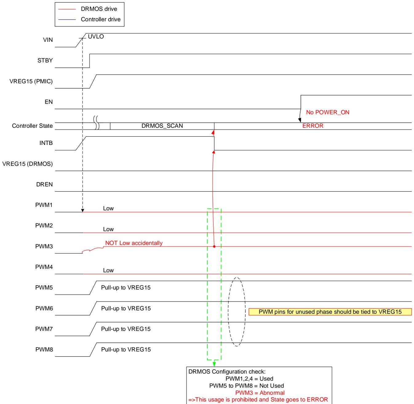
Figure 34. Driver MOSFET Phase Number Scan Example (Error case 1)
