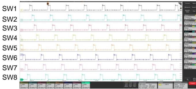
Figure 7. BD9634x series SW Pin Switching Waveform(8phase) (VIN = 5.0 V, Ta = 25 °C)
