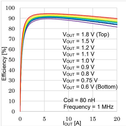
Figure 17. Efficiency vs  $I_{OUT}$  (w/o DCR loss)(VIN = 3.3 V, Ta = 25 °C)
