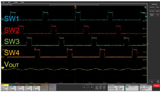
Figure 12. BD9634x series SW Pin and Ripple Voltage(4phase) (VIN = 5.0 V, Ta = 25 °C)
