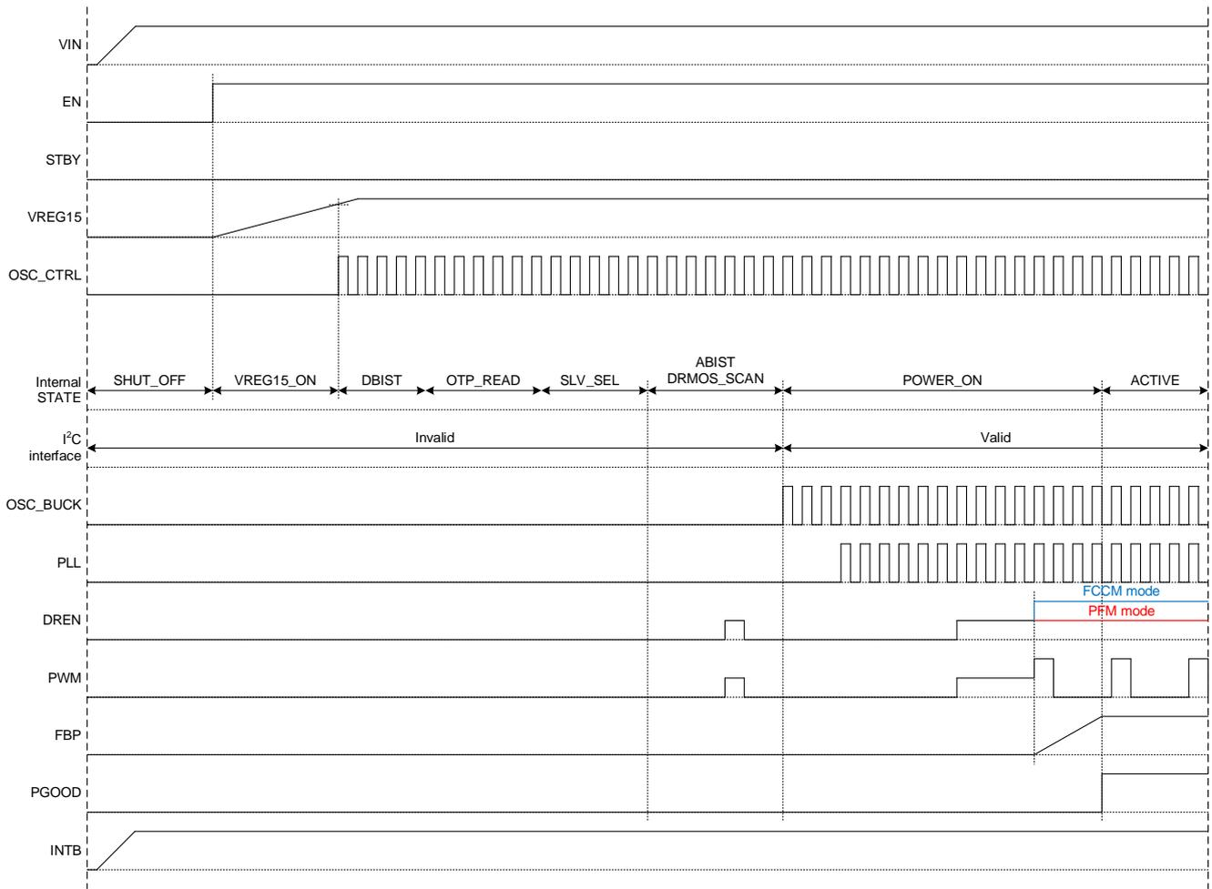
Figure 20. EN ON (STBY OFF) Sequence Timing Chart
