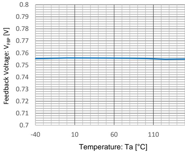
Figure 6. Feedback Voltage (8phase) vs Temperature ( $V_{IN} = 5.0\text{ V}$ )
