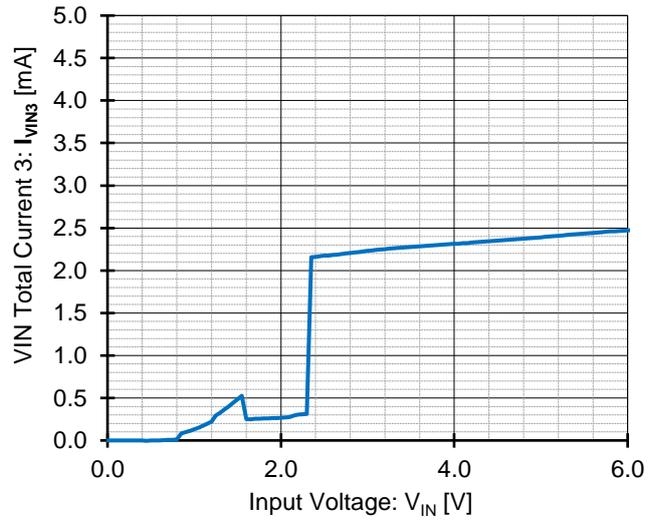
Figure 4. VIN Total Current 3 vs Input Voltage 1 ( $T_a = 25\text{ }^\circ\text{C}$ )
