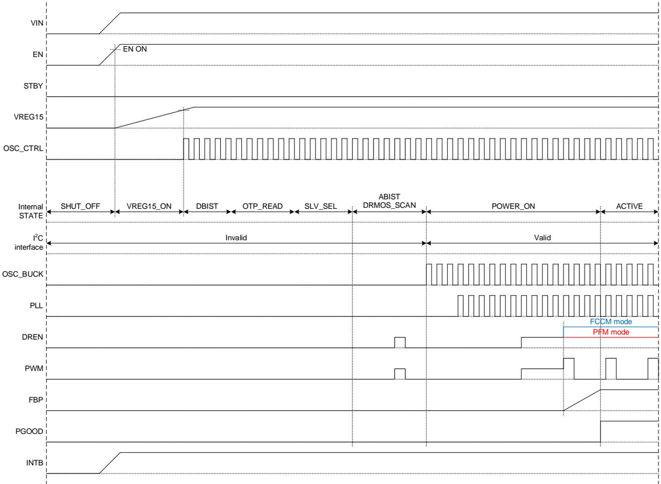
Figure 24. VIN, EN ON Sequence Timing Chart
