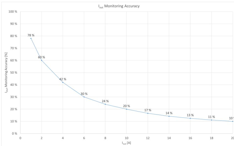
Figure 39. I<sub>OUT</sub> Monitoring Accuracy
