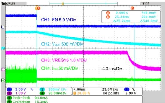
Figure 11. Shutdown Waveform
