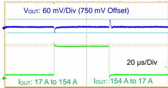
Figure 8. Load Transient (8phase) (VIN = 5.0 V, Ta = 25 °C)
