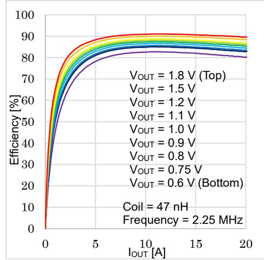
Figure 16. Efficiency vs  $I_{OUT}$  (w/o DCR loss)(VIN = 5 V, Ta = 25 °C)
