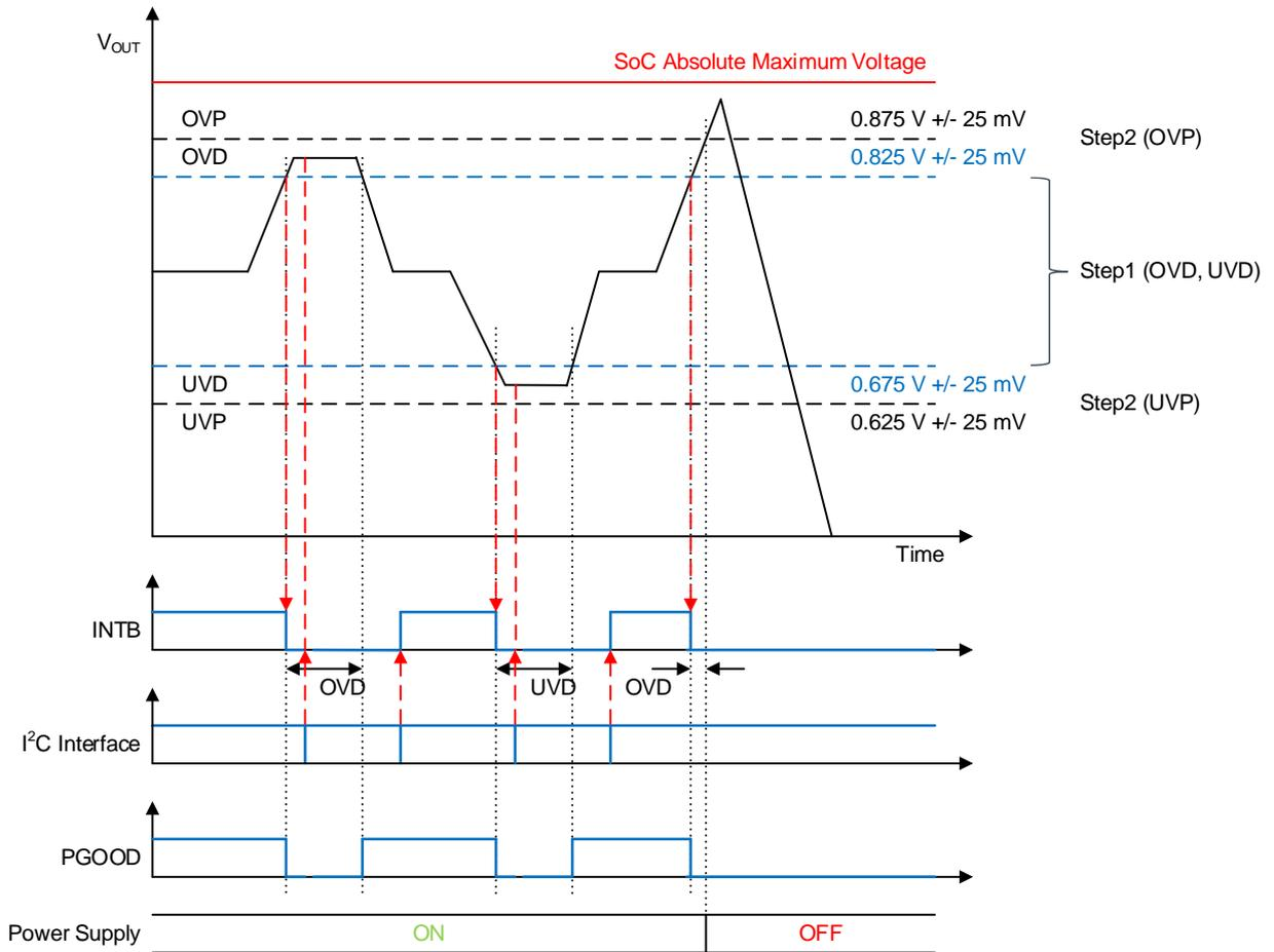
Figure 37. Timing Chart of Voltage Detection Function
