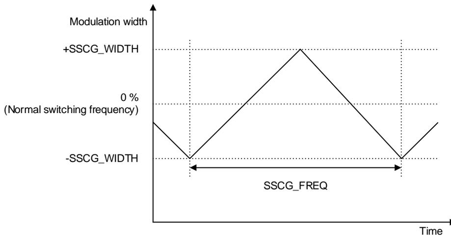
Figure 27. Modulation Waveform of SSCG
