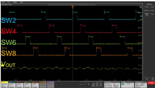
Figure 14. BD9634x series SW Pin and Ripple Voltage(8phase)2/2 (VIN = 5.0 V, Ta = 25 °C)
