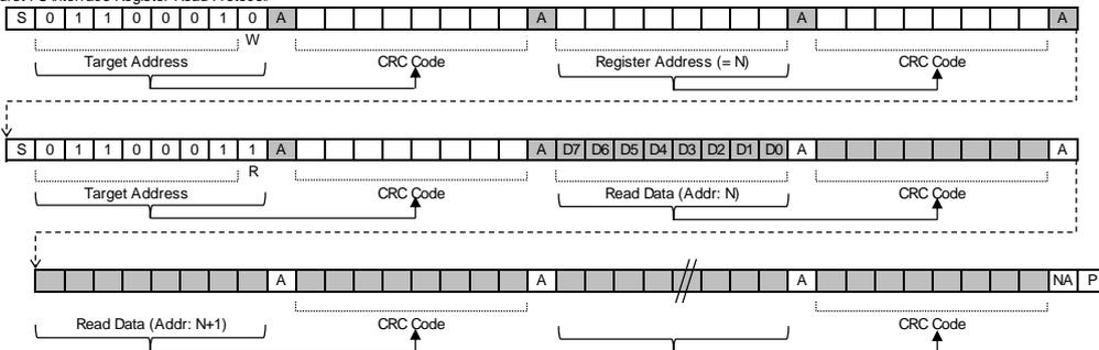
Figure 31. I<sup>2</sup>C Protocol Access of CRC (Example of Target Address: 0x31)
