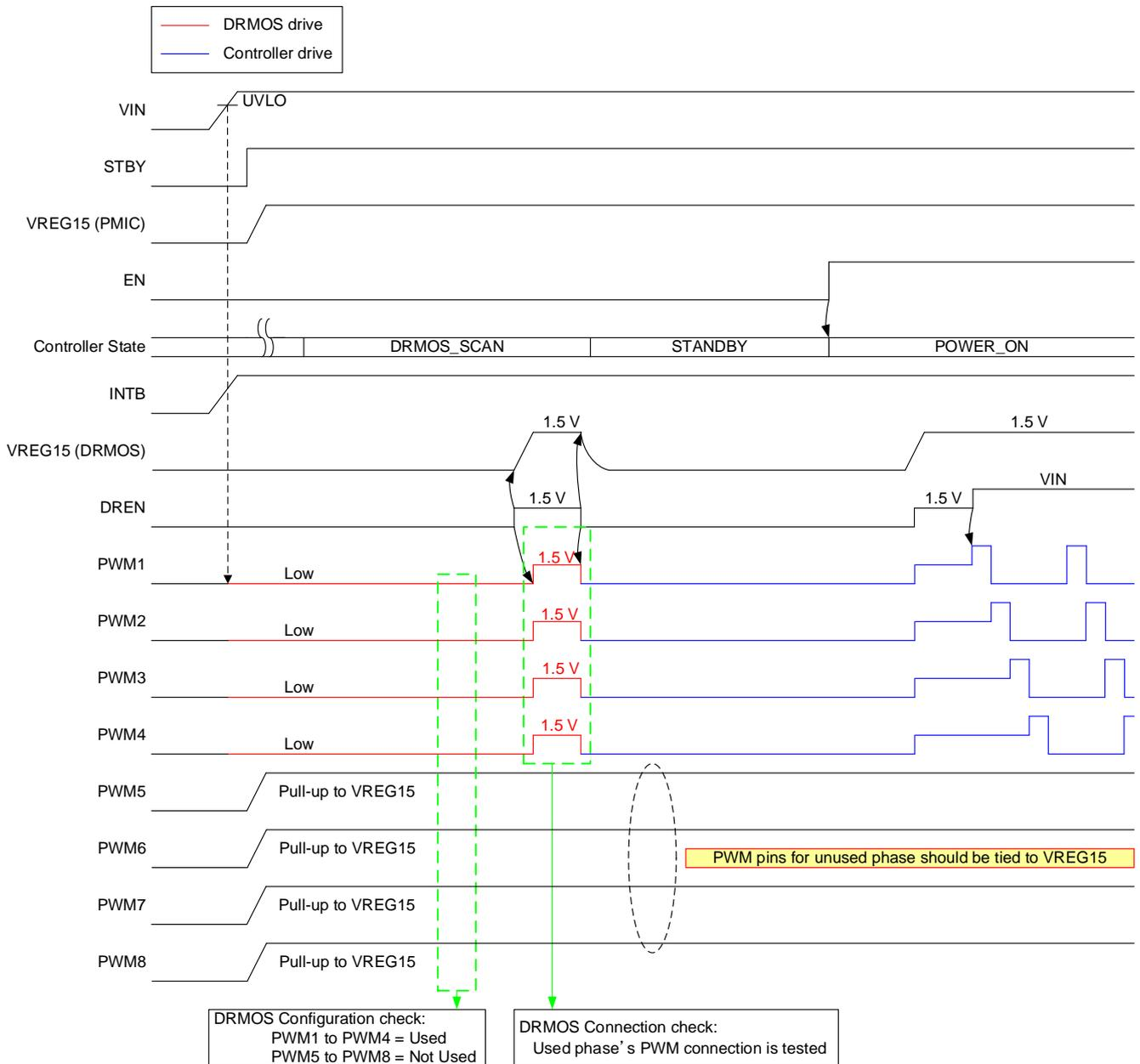
Figure 33. Driver MOSFET Phase Number Scan Example (Normal case with 4 phase)
