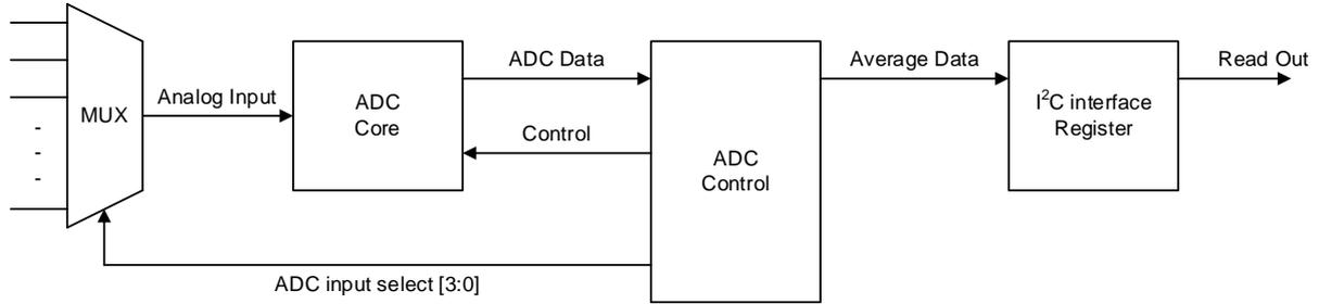
Figure 40. ADC Block Diagram
