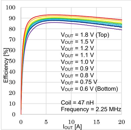
Figure 15. Efficiency vs  $I_{OUT}$  (w/o DCR loss)(VIN = 3.3 V, Ta = 25 °C)
