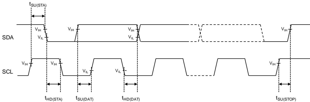
Figure 29. Definition of timing of I<sup>2</sup>C interface
