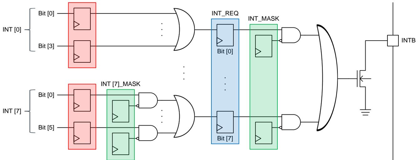
Figure 32. Block Diagram of INTB, INT\_REQ and INT [X] (X = 0 to 7)
