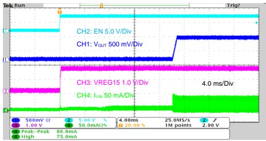
Figure 9. Soft Start Waveform (VIN = 5.0 V, Ta = 25 °C)
