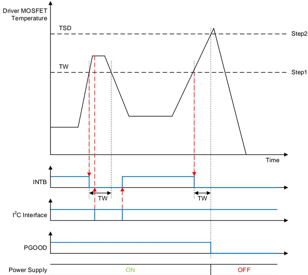
Figure 38. Timing Chart of Thermal Detection Function
