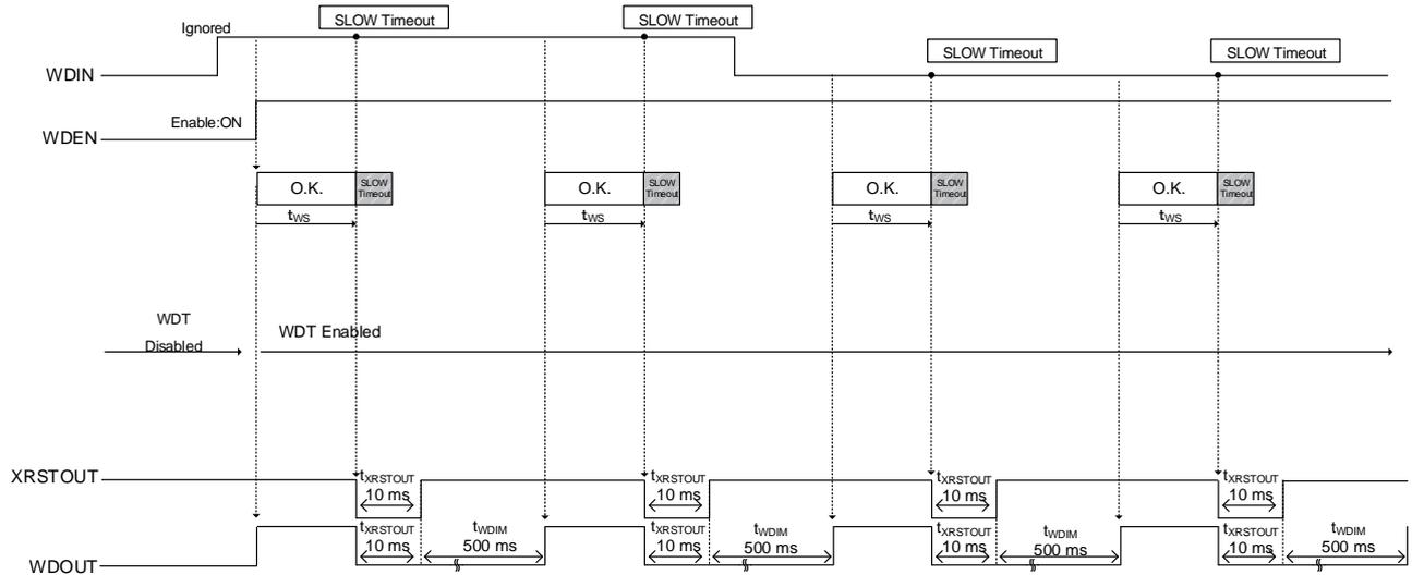
Figure 4. XRSTOUT Behavior with Continuous WDT Timeout Detected
