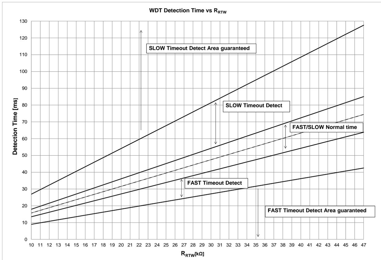
Figure 5. Detection Time vs  $R_{RTW}$
