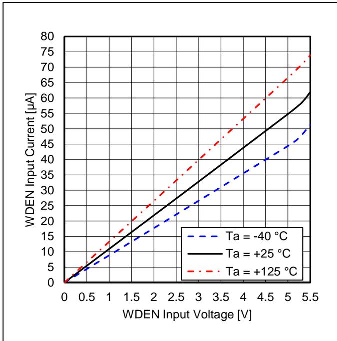
Figure 20. WDEN Input Current vs WDEN Input Voltage ("WDEN Pull-down Resistor Value", V<sub>DD</sub> = 3.3 V)
