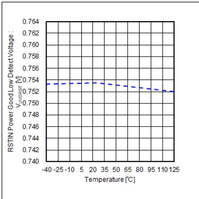
Figure 8. RSTIN Power Good Low Detect Voltage vs Temperature ("RSTIN UVD", V<sub>DD</sub> = 3.3 V)
