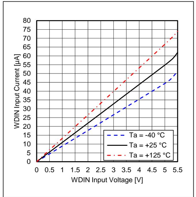
Figure 19. WDIN Input Current vs WDIN Input Voltage ("WDIN Pull-down Resistor Value", V<sub>DD</sub> = 3.3 V)
