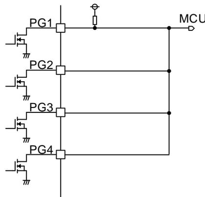
Figure 27. PG1, PG2, PG3, PG4 OR Output
