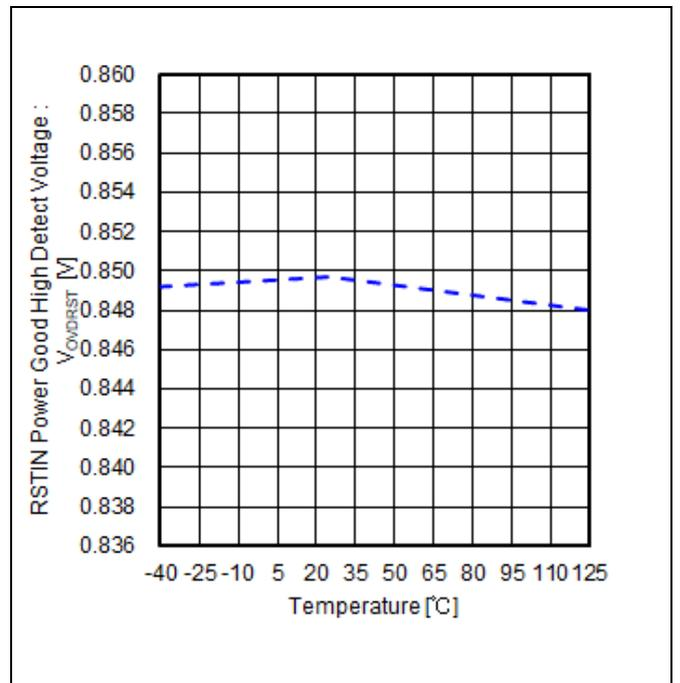
Figure 9. RSTIN Power Good High Detect Voltage vs Temperature ("RSTIN OVD", V<sub>DD</sub> = 3.3 V)
