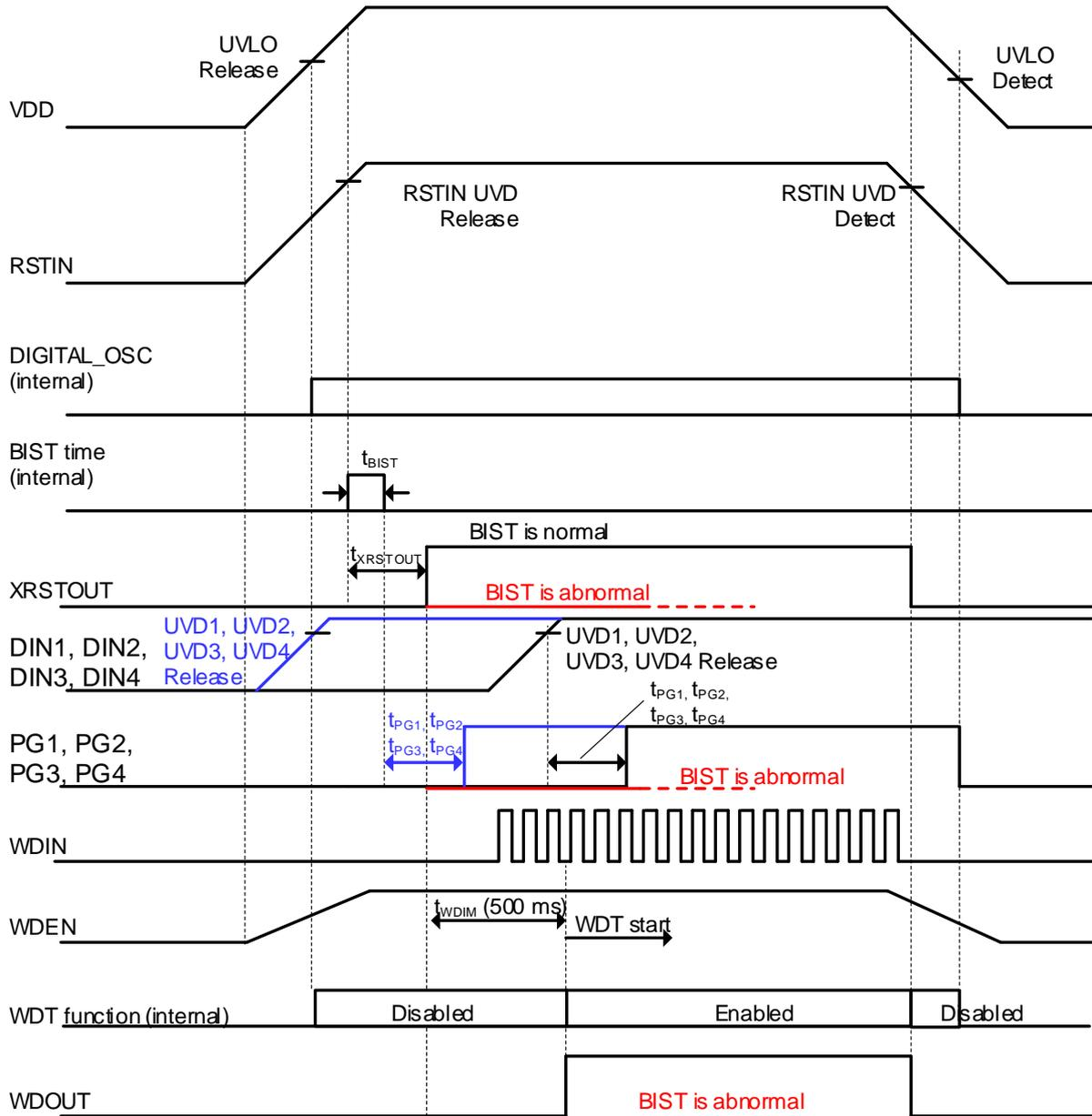
Figure 22. Power ON/OFF Sequence (WDEN is externally pulled-up to VDD)
