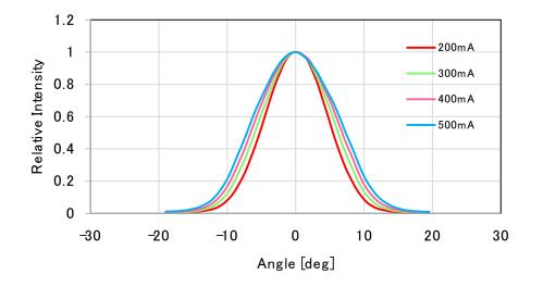
Condition : PKG individual piece , Pulse 50kHz Duty50% (on time 10µsec.)
