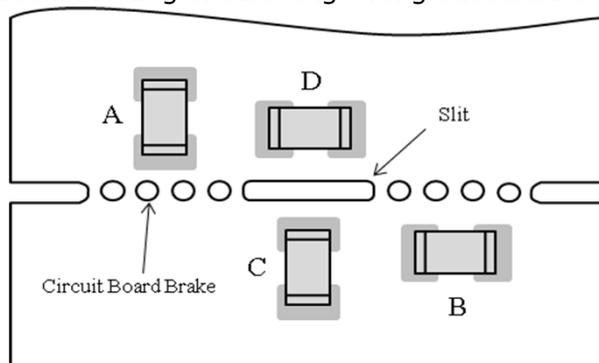
Stress strength according to the mounting position:
