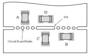
Stress strength according to he mounting position: A > B > C > D
