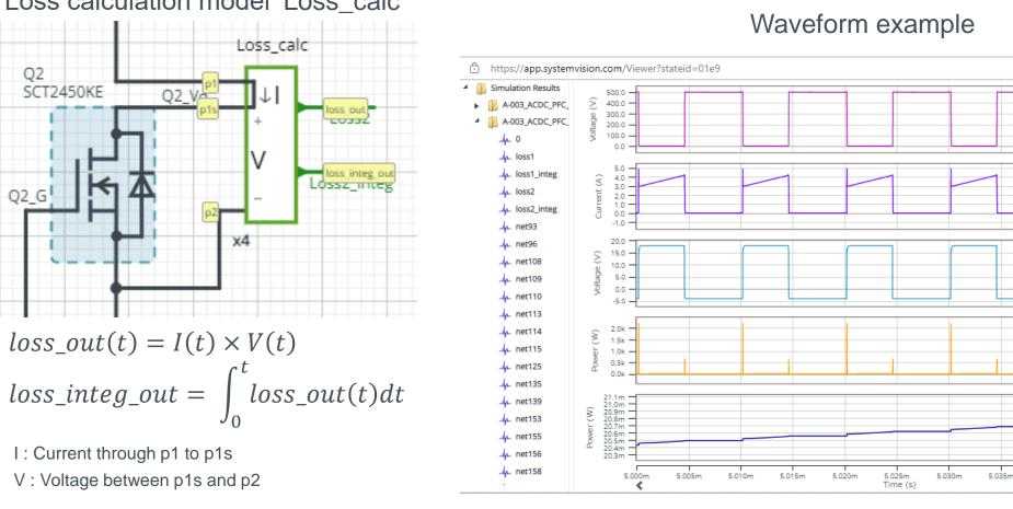
Loss Calculation Model outputs the instantaneous value of power loss and its integration.
