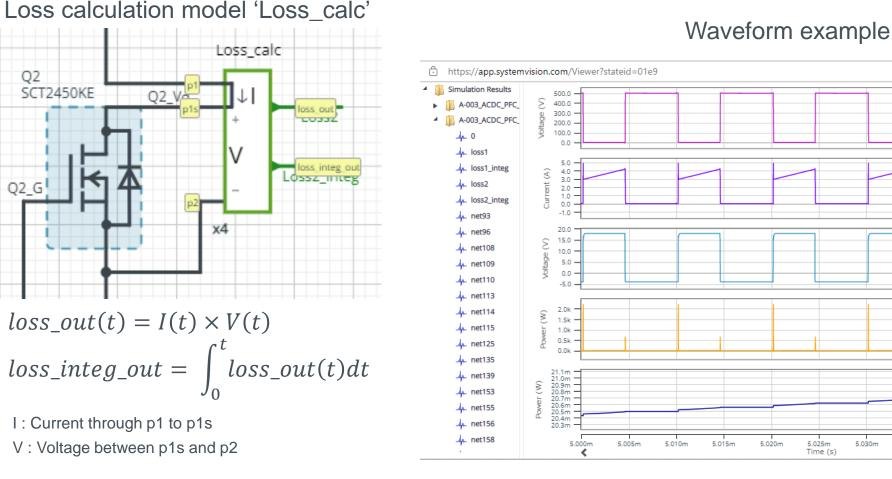
Loss Calculation Model outputs the instantaneous value of power loss and its integration.
