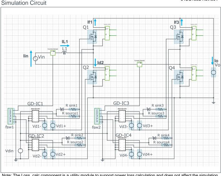
Note: The Loss\_calc component is a utility module to support power loss calculation and does not affect the simulation results of circuit operation or performance. P. 1
