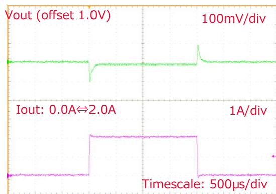
Figure 35 Load response of DCDC_P3V_S1V0
