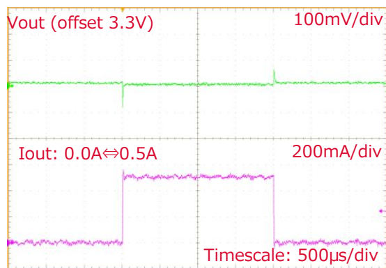
Figure 34 Load response of LDO_P5V_S3V3
