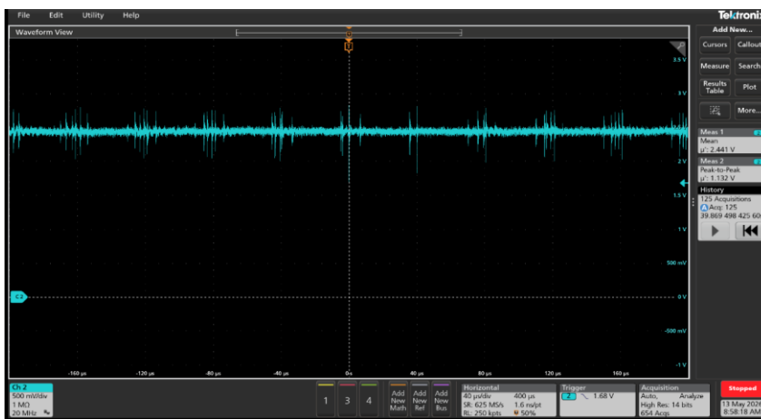
Figure 9. DC bus voltage sensing output measured at sensing board
