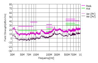
Figure 3. Radiation Noise (vertical antenna)
