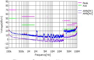
Figure 5. Conduction Noise
