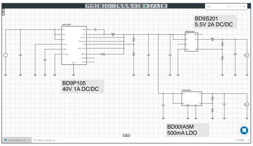
Figure 6. two rails power tree simulation circuit (1)
