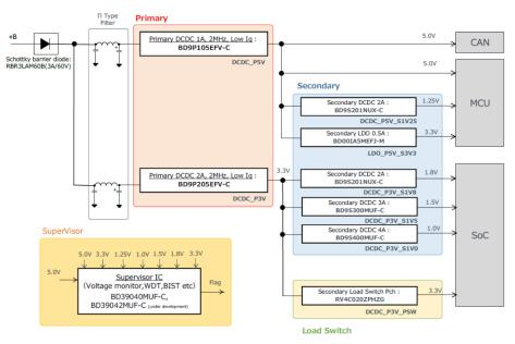
Figure 2. Reference Design (REFRPT001) Block Diagram
