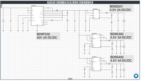
Figure 7. three rails power tree simulation circuit (2)
