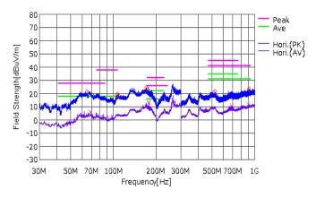
Figure 4. Radiation Noise (horizontal antenna)
