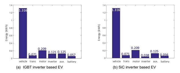
Fig. 11: Comparison of energy consumption under CLTC-P condition
