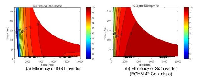
Fig. 6: Efficiency comparison of IGBT and SiC inverter based on simulation (750V)
