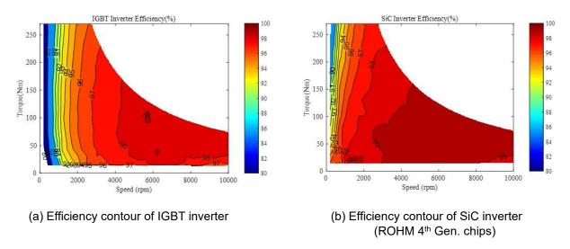
Fig.5: Comparison of testing efficiency between IGBT and SiC (750V)
