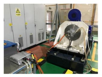
Fig. 4: Efficiency test of SiC motor controller
