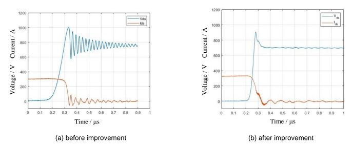
Fig. 2: Turn off voltage and current waveforms before improvement (left figure) and after improvement (right figure)
