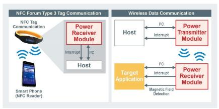
Figure 4. Wireless Data Communication Methods
