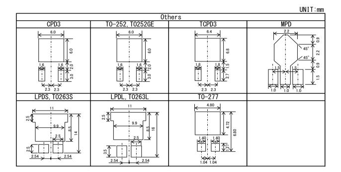
\*Copper plate area dimensions are reference dimensions with being soldered with conditions bellow.
