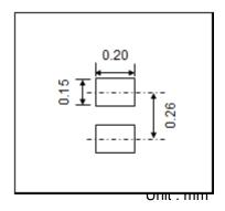
X Copper plate area dimensions are reference dimensions with being soldered with conditions bellow.
