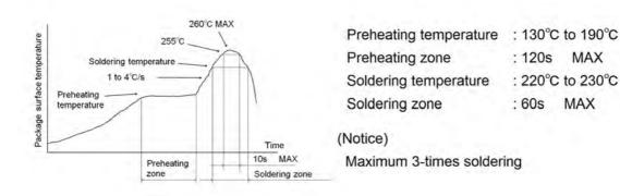
7.2. About mounting with Sn-Pb solder paste
