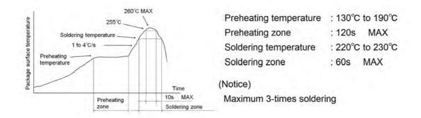
7.2. About mounting with Sn-Pb solder paste
