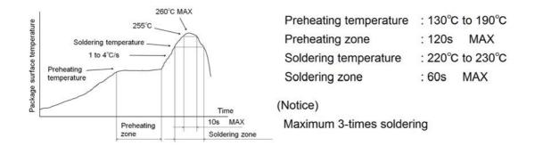
7.2. About mounting with Sn-Pb solder paste
