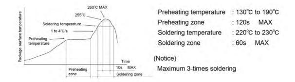
7.2. About mounting with Sn-Pb solder paste
