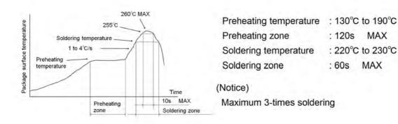
7.2. About mounting with Sn-Pb solder paste
