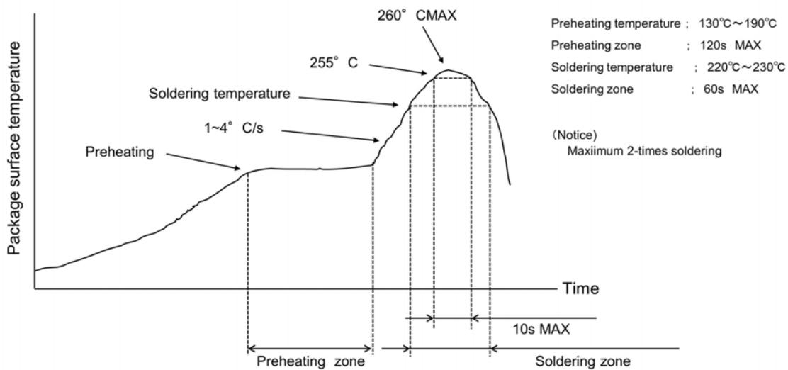
7.2 Recommended condition for wave soldering
