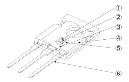
A direction of wire bonding and die bonding, a shape of frame, die size and the number of wires differ by P/N.
