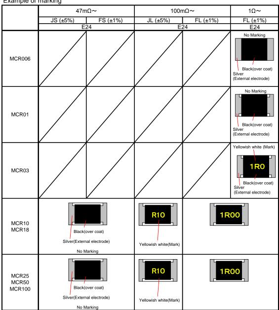
① Marking method: There are three or four digits used for the calculation number according to
