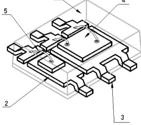
A direction of wire bonding and die bonding, a shape of frame, die size and the number of wires differ by P/N.
